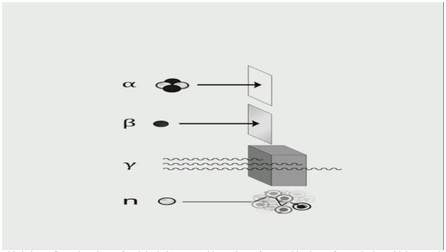
This is just a figurative picture for alpha being stopped by a piece of paper, thin sheet of paper be by a thicker metal, gamma by a solid and neutrons by any other absorption in any other material.
