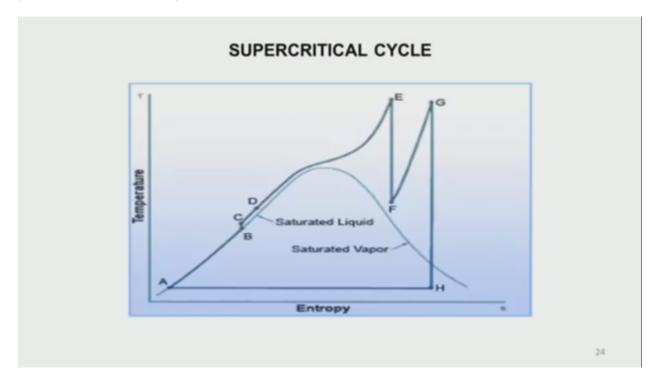
And now this is the cycle, how the supercritical cycle, water entry, pumped in, that's all, becomes -- it becomes steam, then expansion in the high-pressure turbine, coming out, expands, then again heated up to the higher temperature, again coming back and do. This reheating, of course, is there in fossil fuel boilers. Reheating in nuclear reactors is not done because the liquid has to go back into the reactor. So we may have only this portion.
