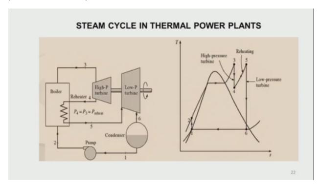
This is just to give you a quick idea about how the cycles are. This is the Rankine cycle, which is normally used in power plants. The water is pumped, sent to the boiler, picks up the heat, becomes superheated, becomes steam, works in the turbine, high-pressure turbine, then comes out, again reheated in the steam boiler, and then comes out and then goes.
