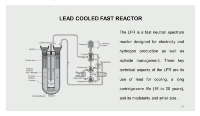
Then the Lead cooled fast reactor. Surely, being a fast reactor, this also has got a very good actinide management so that actinides produced use -- produced in the light water reactors are utilized and broken into short-lived, and so you are able to have lesser waste, lesser activity.
