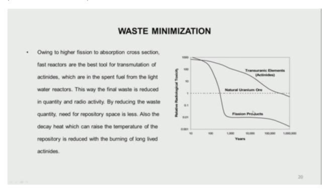
So this is to tell you about the waste minimization as I mentioned. Suppose you don't use fast reactors. You have just an open fuel cycle. See how the actinides will decay to natural Uranium ore level will take many years, over 100,000 years, but the same thing if you had used it in a fast reactor and closed, you reprocess it and use it in a fast reactor, it comes down below within about 100 to 200 years.
