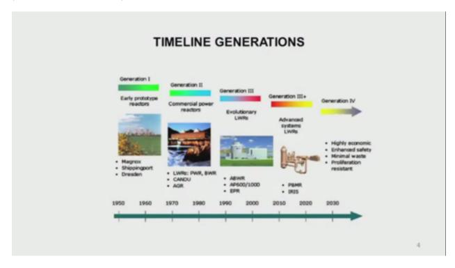
Then the advanced gas cooled reactors, which were improvement over the Magnox reactors. Then there have been some evolutionary designs which have called as the Generation III which took place in the 1990s, the advanced port reactor. Then the AP600 and 1000 reactor designs and of course the European pressurized reactor, which is again was a evolutionary design. It is supposed to be about 1600 megawatt electrical and one of them is under construction in Europe.
