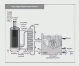
VHTR is to produce both electricity and hydrogen. The reference system consists of a helium-cooled, graphite-moderated, thermal neutron reactor. Electricity and hydrogen are produced using an indirect cycle. Process heat also could be provided for applications such as coal gasification and cogeneration.
