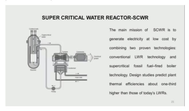
This is a super critical water reactor. As I mentioned, it generates steam at very high pressures and high temperatures, and this technology is a combination of the light water technology with super critical fossil fuel boilers, and efforts are still, of course, in India still we have to build a super critical boiler.
