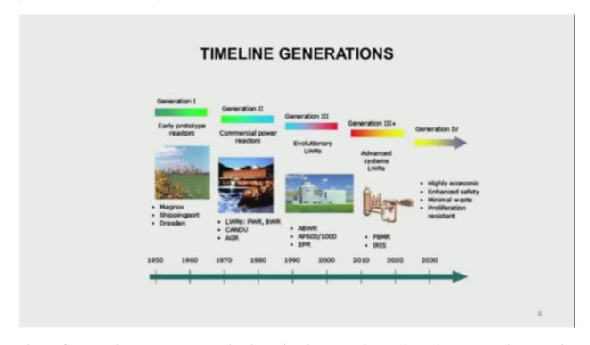
Then, of course, here some more technology developments have taken place. So we have a sub-module Generation III plus. They've got the Pebble Bed, Pebble Bed Modular Reactor development in Africa and then IRIS is another type of reactor design, which has been developed and what is the focus of this Generation IV reactors? Main thing is economics, but enhance the safety. Of course, two objectives. Not that safety is not costly, but safety need not be made excessively costly.
