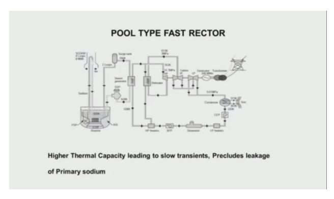
In the pool type reactor, the difference is very simple. We have put all the primary components in a big pool. This is the core. We have the intermediate heat exchanger. We have the pump here which pumps into the core that goes to the HX and comes out to the cold pool. The whole thing is in a single vessel and rest of the circuits are same.
