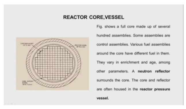
And this whole setup itself is put in a large vessel, steel vessel called as a reactor vessel and of course, it is also a pressure vessel because it has to withstand the pressure of the fluid. So this is a brief idea about what a reactor fuel, a fuel pin, a fuel assembly, or a core or vessel will contain.
