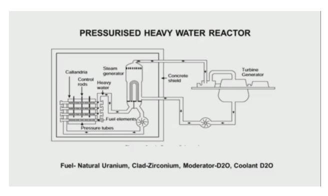
Then this pressurized heavy water reactor. This is our mainstay of India's power program. We have nearly 22 such reactors, most of them about producing about 200 to 220 megawatt electrical each, and some of them are now producing 500 megawatt electrical and we are building heavy water reactors, which can produce 700 megawatt electrical.
