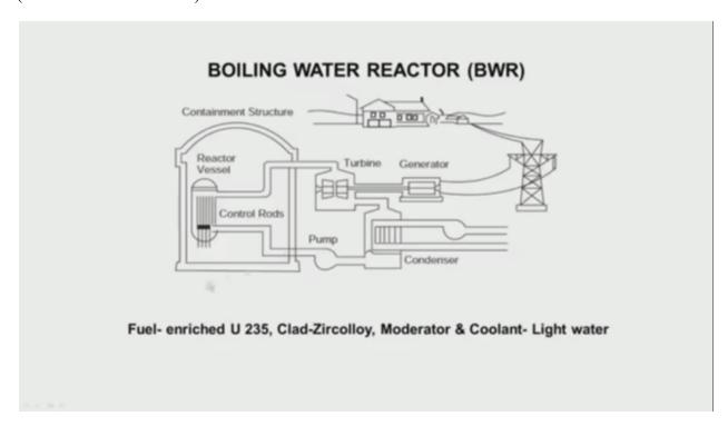
Whereas in a boiling water reactor, steam is produced here and not a full saturated steam. So, and you cannot send the steam mixed with water to the turbine. So you have moisture separators at the top of the reactor, and then only the steam is sent here. Since the moisture separators are here, it puts an obstruction for the control rod. So the control rods are pushed from the bottom. Control rods in a boiling water reactor come from the bottom. This is the difference between the two.
