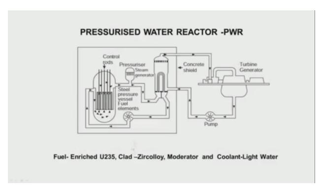
You notice one difference between the pressurized water reactor. Here the control rods are coming from top. The reason is here in this system, everything is water in this. There is no steam at all. It is all water.
