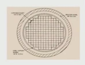
Fig. shows a full core made up of several hundred assemblies. Some assemblies are control assemblies. Various fuel assemblies around the core have different fuel in them. They vary in enrichment and age, among other parameters. A neutron reflector surrounds the core. The core and reflector are often housed in the reactor pressure vessel.
