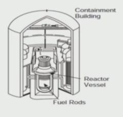
All the components of the reactor are contained in a solid concrete structure that guarantees further isolation from external environment. This structure is made of concrete that is one-meter thick, covered by steel. The most recent reactors sometimes contain two containment structures and are designed for the impact of an aircraft.
