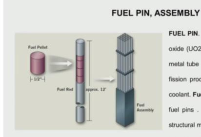
FUEL PIN. These are typically uranium-oxide (UO2). They are surrounded by a metal tube (called the cladding) to keep fission products from escaping into the coolant. Fuel assemblies are bundles of fuel pins. The assemblies have some structural material to keep the pins close but giving room for coolant to flow.
