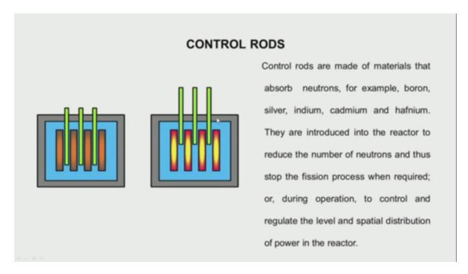
Now if I want to control the power, I will reduce the height, bring it inside and maintain it at level. The neutron population will come down and then stabilize at another level. Then that way my power would have been brought down. If I want to increase the power, I slightly rise one by one. Not all rods are raised. Only one by one at a time.
