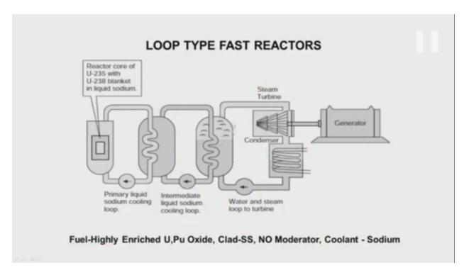
So we have an intermediate circuit. This is designed to withstand the pressures of a sodium water reaction. So that is a reason why we have two such circuits. They as I mentioned enriched Plutonium, Plutonium oxide is a fuel. Clad is stainless steel. No moderator and coolant is Sodium.
