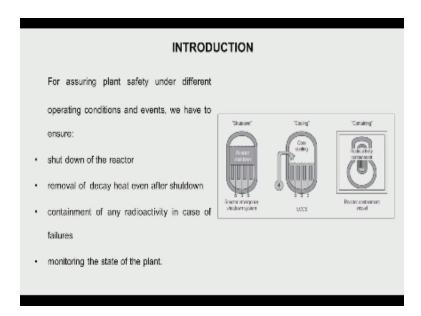
First in case, of an event we must be able to shutdown the plant. Maybe we should assure a safe shutdown of the plant. When, we do this shutdown we have stopped the fission reaction. The chain fission reaction has been stopped. But still heat is getting produced in the reactor due to the decay of the fission products.
