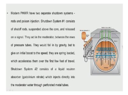
We have the shutdown system one which has these control rods here you can see some control rods moving then we have the other shutdown system which consists of gadolinium nitrate
