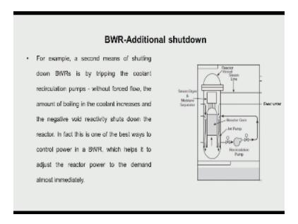
In the case of the boiling water reactor it is you know it is very sensitive to temperature the reactivity. Is very sensitive to temperature and if the inlet temperature through the reactor. Increases then your wide generation will be more and you know most of the designs. We have negative reactivity worth of the boiling water reactors while because of boiling there is a negative reactivity and the power comes down.
