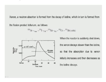
How this xenon is produced of course tellurium one of the fission products it decays with the one minute time constant or decay constant becomes iodine 135 again with the 6.7. Our decay constants becomes xenon 135 which after a decay of 0 is the concept of 19.2 hours. Become cesium and finally barium so there is a always when the reactor starts there is an increase of the xenon then after sometime. There is an equilibrium situation and when you shut down again it comes down.
