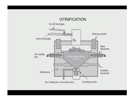
This is just to give a figure of the process. This process is called the verification. There is mixing glass and the fuel, high level waste and then trying to make this thing. So the glass is molten at about 1200\* centigrade and we add the waste high level waste and then we pour it and then make it into a solid form and this solid form we put in radiation shielded casks and put it under the ground.
