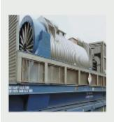
Spent fuel and high-level waste, are highly radioactive and require special handling. To limit the risk in transporting highly radioactive materials, containers known as spent nuclear fuel shipping casks (Fig.) are used which are designed to maintain integrity under normal transportation conditions and during hypothetical accident conditions.
