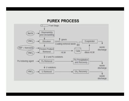
There is a process which is a well known Purex Process which is used in reprocessing and just to get an idea, what is the components of the Purex Process you can have a look at this figure, it's a schematic figure in which involves the disassembly of the fuel, the decladding, remove the cladding material of the fuel, then dissolve it using nitric acid, then to extract the fission products they use TBP plus Kerosene, It is Tributyl phosphate and Kerosene along with nitric acid then
