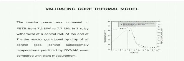
So what we did, we raised the power of the reactor from 7.2 megawatts to 7.7 megawatts in seven seconds by withdrawing the controller rod. At that time the reactor tipped. So this data we had and the central sub-assembly, the centermost sub-assembly, the monitoring of those temperatures were also recorded. So we said okay come on, let us now, why not we use our model to look at this transient event and let us predict. Now this star ones show you what is the
