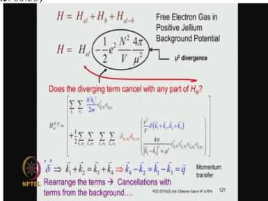
So, this is the picture we had before us. So, we have the electron-electron terms in this part of the Hamiltonian. And then you have the nuclear-nuclear interaction terms which is the interaction between all the positive charges of the Jellium plus the interaction between the electron and the positive charges which are smeared out in the Jellium potential.
