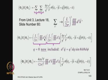
Now this is what we have to evaluate but we are not going to carry out a discrete summation. We are going to carry out an integration in the momentum space right. So, the summation over k goes over to this integration in the momentum space with this factor because of the volume occupied by every state right.
