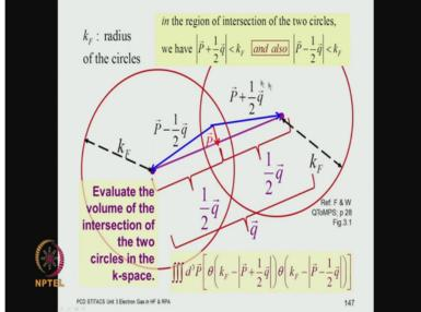
And essentially what it tells us that if you look at this region of intersection of these two circles you have this condition satisfied that P + half q is less than k F and P - half q is also less than kF. So, this carrying out this integration this is the integral that we have to determine.
