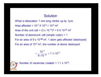
So, we are told that you have an the area is 1 millimetre 10 to the power minus 3 meters into one micron metre, which is 10 to the power minus 6 which is 10 to power minus 9 meters that is the area affected. It is 3 into 10 to the power minus 10 square which is 9
