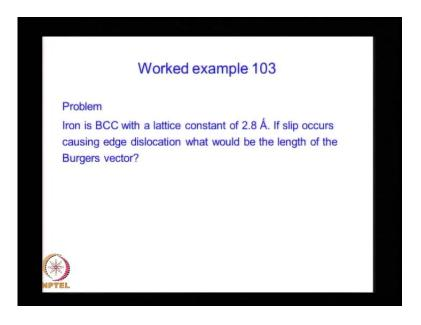
In the last question, we are told that iron has a body cantered cubic structure with a lattice constant. If slip occurs causing edge dislocation what would be the length of the Burgers vector? You know that the slip direction in a bcc structure is 111. And it is a by 2 111. So, this will be in the case of 111, since lattice constant is 2.8 angstroms, this 2.8 into root of 1 square plus 1 square plus 1 square by 2. So, this will be which is...
