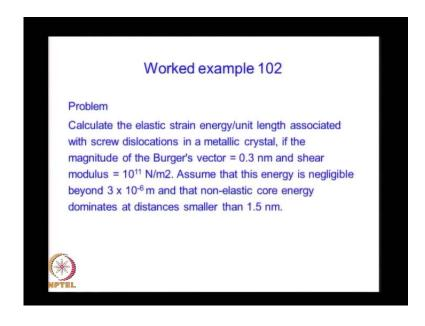
The next problem concerns the elastic strain, we are asked to calculate the elastic strain per unit length associated with screw dislocations in a metallic crystal. We are told that the burgers vector is 0.3 nanometres. The shear modulus is 10 to the power 11 newton per metre square. You are also given as to assume that this strain energy is negligible beyond 3 into 10 to the minus 6 meters, and the non elastic core energy, dominates at a distance less than 1.5 nano meters.
