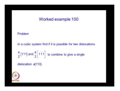
The first example tells us that we have a cubic crystal and we are asked to check if it is possible for two dislocations represented by a by 2 111 each whether it is possible for these two dislocations to combine to form a single dislocation at 110 that is the question, a 110.
