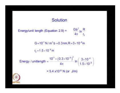
This is the substitutional problem in which we know the expression for the strain energy which was discussed in the lecture it is strain elastic strain per unit length is G b square by 4 pi log R by r zero. So, in this, this is b, this is G this is r zero and this is R. So, substituting these values 10 to the power 11 into 0.3 into 10 to the minus 9 square by ln R is 3 into 10 to the power minus 6 by r zero is 1.5 into 10 to the power minus 9. So, calculation gives per metre.
