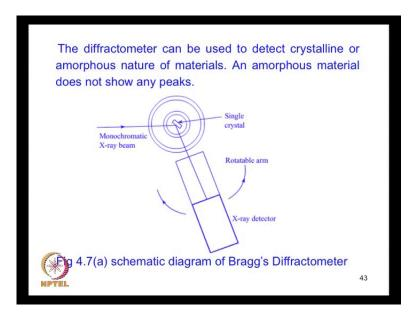
And the next figure shows the experimental arrangement in a Diffractometer. You have the schematic diagram is shown with a monochromatic x- ray beam incident on a single crystal and then the diffracted beam is seen by a interms of using an x-ray detector mounted on rotatable arm the diffraction . So, the x-rays get Bragg reflected from various crystal planes in different directions the x-ray detector shows a peak at those angles at which the Braggs law is satisfied by a set of crystal planes.
