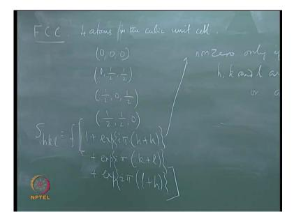
We see that there are four atoms in the unit cell, cubic unit cell. one at 0, 0, 0 then one at 0, half, half at the face center, one at half, 0, half and another at half, half, 0 these are the coordinates of the centers of the faces. So, the s h k l in this case is going to be f times 1 plus exponential i pi into h plus k plus exponential i pi into k plus l plus exponential i pi into l plus h.
