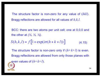
A body centered cubic lattice has two atoms per unit cell one atom at 0, 0, 0 and another one atom in the body center of the cube, which is half, half, half inside the distance of half the lattice separation the distance between consecutive atoms. So, substituting this you get s h k l equals one plus f times one plus exponential i pi the 2 pi cancels with the two factor 2 cancels the 2 in the denominator.
