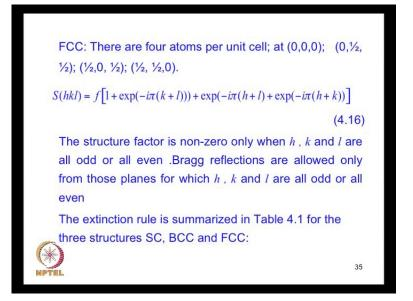
So, the structure factor will be nonzero in this case only when this will be nonzero only when h k and l are all odd or are all even. So, that is the extinction rule for a face centered lattice.
