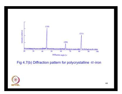
So, such a diffraction pattern for iron is shown in figure can see the diffraction maxima the Bragg diffraction maxima corresponding to different h k l planes. When the intensity of the scattered x-ray is plotted as a function of the diffraction angle. So, we have now, considered all the important techniques of x-ray diffraction.
