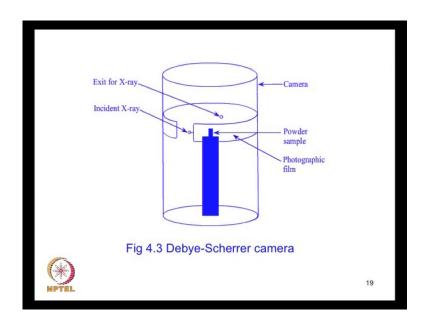
So, that is the Debye Scherrer camera and you see the sample mounted at the center. A strip of photographic plate is positioned inside the camera around the inner wall. So, you have a strip positioned around the inner wall of this camera. So, there is a photographic film. In the middle such that the films surrounds the sample, the camera has a hole for the incident x-ray and a diametrically opposite hole for the outgoing x-ray. So, there is an entrance for the incident x-rays and an exit.
