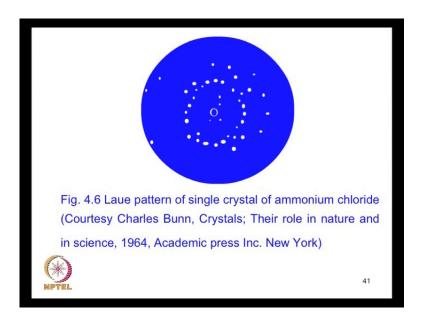
So, the next figure shows a Laue pattern for a single crystal of ammonium chloride. So, you see how the diffraction spots are distributed.
