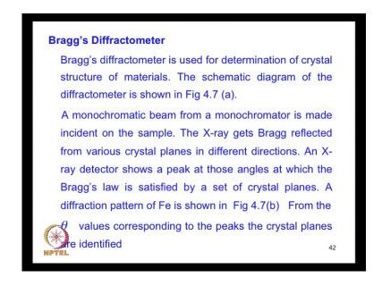
The third method goes by the name the Bragg Diffractometer this is the bread and butter of every x-ray crystallography. This is used for the determination of crystal structure of materials. (Refer Slide Time: 46:18)
