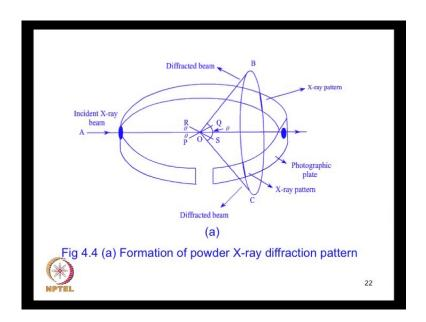
So, from this figure you can see that the solid angle subtended by the cone is 4 theta. So, each set of planes for a given specific h k l value gives rise to a such a cone of reflected rays and therefore, these cones intersect the cylindrical photographic plate in circles as illustrated in the next figure.
