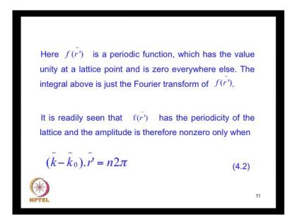
So, this is a, this f of r prime is a periodic function depending on the distribution of atoms. So, it has a maximum value at the site of a lattice point it is unity and it is zero everywhere else where ever there is an atom there is scattering amplitude. So, it has this has which has the same periodicity is the same as that of the crystal lattice. So, it has the same thing therefore, this amplitude will be nonzero.
