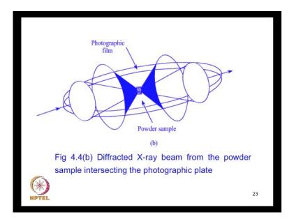
So, these cones intersect the photographic plate. So, you have the diffracted x-ray beam from the powder sample intersects the photographic plate. So, you get each cone generates a pair of arcs on the photographic plate. The arcs are positioned symmetrically
