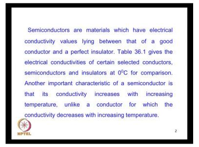
Unlike whereas, semiconductor conductivity increases, so this is called a positive temperature coefficient. So, this has a positive temperature coefficient of resistance. So, this is known as ptc. Whereas, the metals is known as ntc, it has a negative temperature coefficient. So, this is another important difference between the behavior way temperature variation of the conductivity of a semiconductor versus that of a metal.
