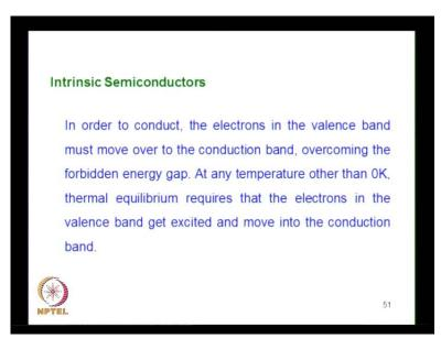
Now if you want to understand the nature of conduction in a quantitative manner, we have two discuss a in terms of for an intrinsic semiconductor will go by carrier concentration, how to determine the carrier concentration in an intrinsic semiconductor.
