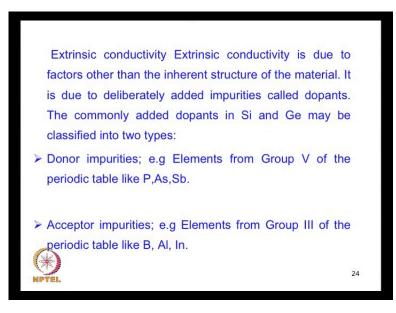
Now, the impurities can be of two types. The impurities which are added can be either donor impurities or acceptor impurities. A donor impurity is one which donates an electron for example, an element from group 5 in the periodic table, we already saw these elements like phosphorus, arsenic and tumanic; whereas, acceptor impurities are one which are from an element from group 3 such as bismuth, aluminum, indium. So, these are added in extremely small quantities in at the part per million.
