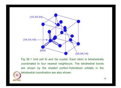
So, figure shows the unit cell of silicon and germanium crystal. In this, we will discuss this in great detail, but this is the main feature. Each atom of silicon is tetrahedrally coordinate, have a cube and each atom of silicon is tetrahedrally coordinated, auto four near neighbor - tetrahedrally coordinates. Tetrahedron means the near neighbor is 4. So, each silicon is coordinated to 4 near neighbor silicon. So, there are tetrahedral bonds which are shown by shaded portions.
