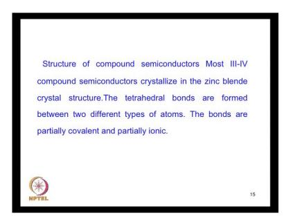
This is also the case with most compounds semiconductors, the compound semiconductors are formed by combining a group three element with a group five element or a group two element with a group six element.
