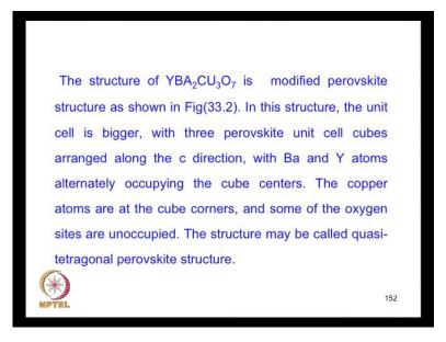
And the three cubic unit cells are stacked along the axis with the barium and yttrium atom alternately occupying the body centers of the cube. The copper atoms are at the cube corners and some of the oxygen sides are not occupied. So, it is a kind of quasi tetragonal perovskite structure which is a laid structure with alternating copper oxygen ion layers and barium or yttrium oxygen ion layers. The copper oxygen ion layers form conducting layers. (Refer Slide Time: 32:45)
