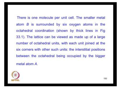
So, you have the lattice which can be viewed as being made up of a large number of such octahedral units with each unit joined at the six corners with other such units at the six corners of the octahedral and the interstitial positions between octahedral are occupied by the bigger metal atom a. So, that is the basic cubic structure now the yttrium barium copper oxide is a modified version of this.
