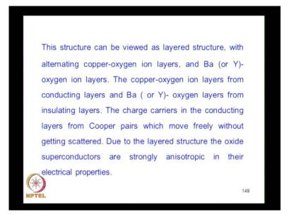
So, you have a kind of quasi two-dimensional charge transport, these copper atom are responsible for the superconductivity. The barium or yttrium oxygen layers form insulating layers between this conducting playing is the charge carriers in the conducting layer form upper pairs which move freely without getting scatter. Due to the layer structure the oxide superconductors are strongly anisotropy. So, that is the basic crystal structure.
