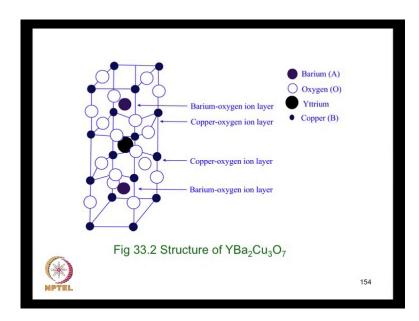
Now, this is shown in the next figure. Now you have a modified version in which we are showing the unit cell is bigger with three perovskite you read the cubes arranged along the c axis you can see it is tetragonal crystal not a cubic one and you have a c axis like this.
