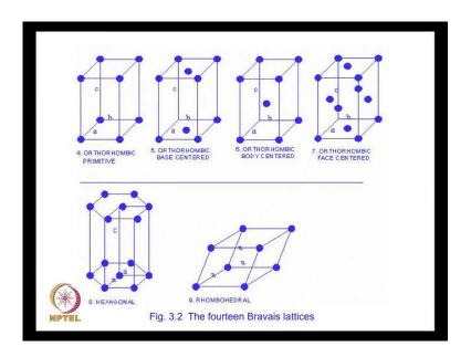
Then the orthorhombic as all possibilities orthorhombic primitive orthorhombic body centred orthorhombic face centred orthorhombic end face centred then you have a hexagonal and a rhombohedral lattice we then come to tetragonal primitive.
