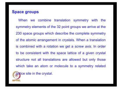
And cubic face centred. So, these are the fourteen lattice types now when we combine translational symmetry with symmetry elements of the 32 point groups we arrive at the two hundred and thirty space groups which describe the complete symmetry of the atomic arrangement in crystals.
