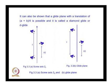
So, you have an atom which is brought into rotation and then translated along the rotation axis, so that is a screw axis similarly shows a glide plane where there is a mirror
