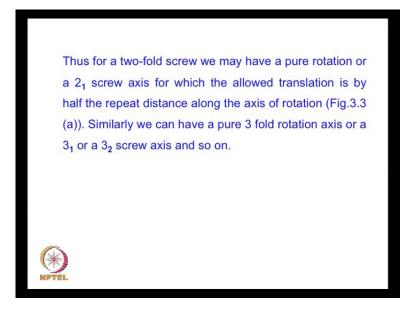
So, for example, for a twofold axis we can have a translation by half the repeat distance along the rotation axis as shown in the next figure.
