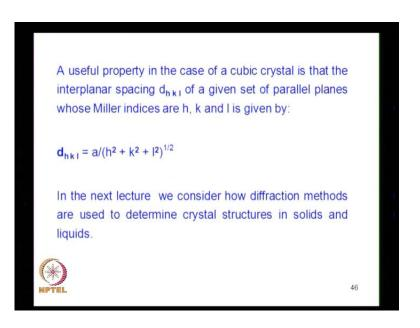
It is one useful property for a cubic crystal is that the inter planer spacing is the lattice parameter divided by h square plus k square plus l square.
