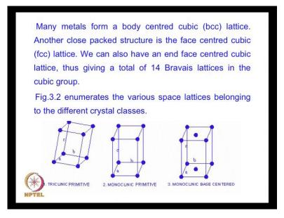
Many metals form body centred cubic lattice others have the face centred cubic lattice or sometimes the end face centred only one pair of end faces gets entered. So, these are the different Bravais lattices and figure shows the various space lattices belonging to the different crystal classes. For example, here we have the triclinic primitive lattice a primitive lattice is one in which there are atoms only at the corners then you have a monoclinic primitive and a monoclinic body centred.
