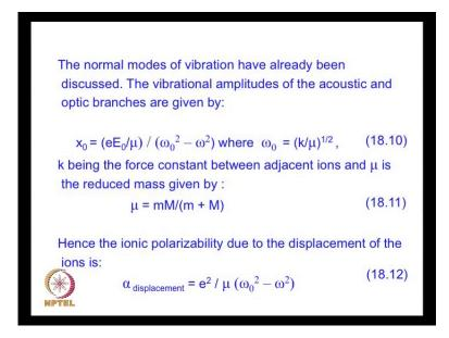
We arrived a situation where x naught to the equation motion and solid salt it and law where this omega naught this k by mu and mu is reduce mass of the two ions given by from this once we know the displacement.
