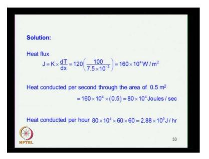
That would work out to be 8 into 10 to the power 4 joules per second.
