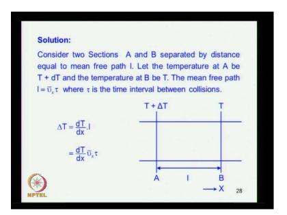
So we consider two sections at temperatures T and T plus delta T, so there is a temperature gradient along this direction, so let us call this x direction. So there is a temperature gradient and let us take these two sections call them A and B. And the mean free path 1 is v x and tau, where tau is the relaxation time or collision time; and v x is the average x component of the speed. Therefore, if this section is separated by a mean free path, then delta t is d T by d x times v x bar tau.
