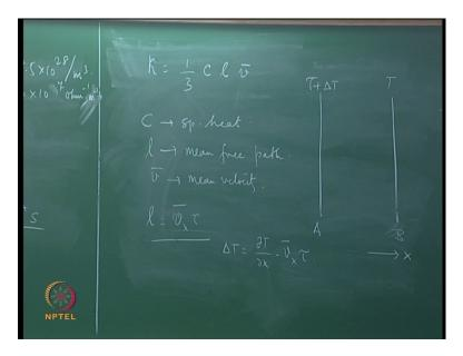
We ask to prove the thermal conductivity the kinetic theory expression of thermal conductivity for a perfect gas as one third C l v bar; where C is the specific heat, l is the mean free path, and v bar is the average mean velocity of the gas molecules. So this is the expression that we will adapt for discussing thermal conductivity of metal as well.
