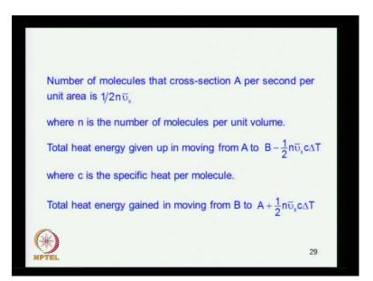
Now we calculate the number of molecules which transport energy thermal energy to the two sections by moving by carrying heat along the x directions.
