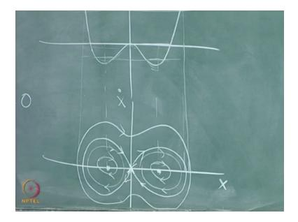
Here is the potential and if I plot X here versus X. for instance on this side then the phase trajectories are very straight forward, you have a little center here you have a center here and you have a hyperbolic or saddle point out there. For small enough energy just above the minimum of this potential you could have stable oscillations about either of these centers and therefore you would have trajectories of this kind for.
