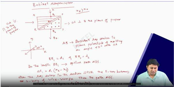
So with this path difference when the light emerges from the system then what happened the resultant phase difference the resultant phase difference will be delta phi and that is 2 pi
