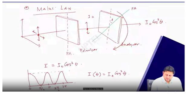
After passing through the polarizer and then if we rotate this another Polaroid film we have and if we rotate this 90 degree. So that its pass axis is now perpendicular to the previous one,
