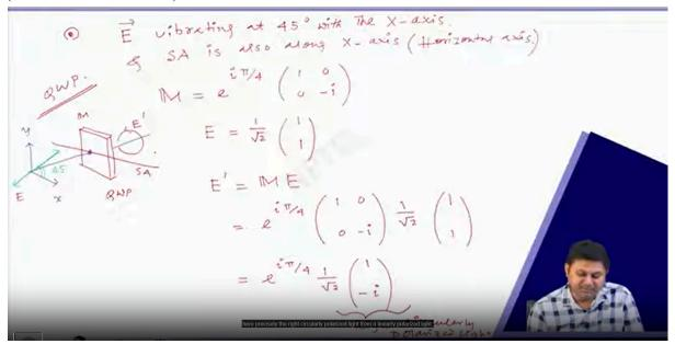
Now the m for this case will be simply e to the power of minus i pi by 2, 1-0-0 minus 1 when SA is vertical and it is operating over this e, which is a plane polarized light that is having an
