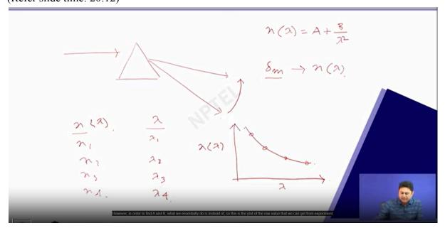
By exposing the prism to white light and then you get a spectrum here, different color and three or four strong color, for three and four strong color you can figure out what is the value
