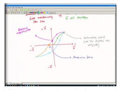
So, it will reduce in this way, so there is a gap here, so this point you can see that even though my magnetic field is 0, I should have some magnetization here still. So, this magnetization is called the residual magnetization. Why residual? Because even though I have my external field 0 the material is still having some sort of magnetization, then what happened? I further reduce, now I need to make it 0, so I further reduce my magnetic field in the opposite direction.
