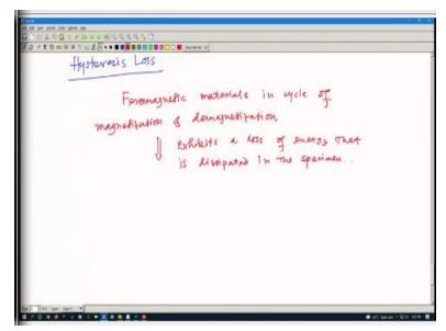
Hysteresis, so what happened that? Ferromagnetic materials in cycle of magnetization and demagnetization, so once it is magnetized and then again demagnetizes, during this process what happened? It exhibits a loss of energy that is dissipated in the specimen itself. So, this hysteresis loss I can calculate in this way.
