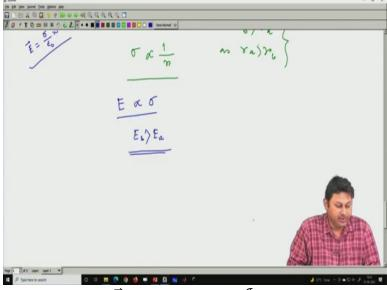
Because we know that electric field  $\vec{E}$  is how much it is  $\frac{\sigma}{\epsilon_0}$  with  $\hat{n}$  this is the vectorial form so that means the electric field is proportional to  $\sigma$ , so, the electric field will be also higher. So, that means, if I want to find out the electric field for these 2 sphere one is say  $E_a$  and another is say  $E_b$  then  $E_a$  so from here we can also write that  $E_b$  is greater than  $E_a$ , this is the condition I should have.
