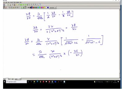
So,  $\frac{\partial \Phi}{\partial r}$  comes up to be  $\frac{\lambda}{4\pi\epsilon_0}$  will be constant and stay like this and I have  $\left[\frac{1}{A}\frac{\partial A}{\partial r} - \frac{1}{B}\frac{\partial B}{\partial r}\right]$ . Now  $\frac{\partial A}{\partial r}$
