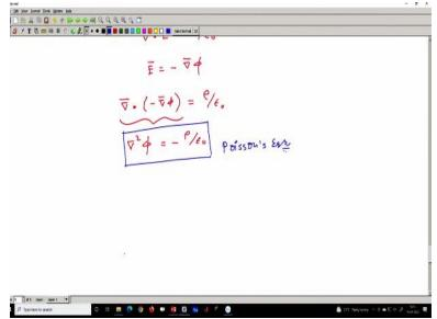
So, if I replace this in the first equation, then I simply have divergence of minus of gradient of the scalar field  $\phi$  is  $\frac{\rho}{\epsilon_0}$  this quantity this is not new, we have already discussed this quantity earlier. This is simply forms the Laplacian, which is  $\nabla^2$ . So, this basically leads to a  $\nabla^2$  operator and I can write it as  $-\frac{\rho}{\epsilon_0}$ . So, this very equation is called the Poisson's equation.
