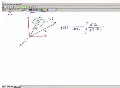
Next, in a similar way if I go on in case 3 for surface charge I have a coordinate system and then I have a small surface element here which we call ds' and like before we have these coordinate points this is  $\vec{r}$  and this is  $\vec{r} - \vec{r}$ , the potential here should be simply  $\phi$  at  $\vec{r}$  for this kind of distribution is  $\frac{1}{4\pi\epsilon_0}$  integration of  $\sigma$ , which is a surface charge density ds' over  $\vec{r} - \vec{r}$ ,
