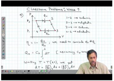
So, of course, we although it is not given in the question here, but it is obvious that heat can enter only in this adiabatic, it is isobaric, isobaric expansion phase and heat may go out of the system only in this isobaric compression phase. So, typically that happens inside a cycle that during the expansion, heat comes in, during the compression heat goes out and of course, these 2 processes are adiabatic. So, there is no heat exchange.
