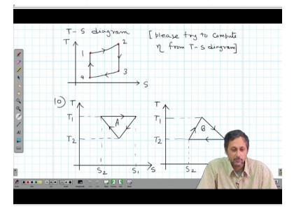
Now comes the T-S diagram part. Now for the T-S diagram, it is actually very simple we have process 1 to 2 which is isobaric where the heat comes in and of course, when the heat comes in the entropy increases, the temperature increases. So, all 3 entropy volume and temperature all 3 increase, we can see air pressure remains constant, we can see volume increase from here. So, this part will be represented by a nonlinear implement of temperature and entropy.
