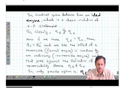
So, what happens in this case when eta E is equal to eta C then Q 2 is equal to Q 2 prime. So, in this case what happens is it will be completely 0, this Q 2 minus Q 2 prime in this both cases, so the combined system will not accept any heat from any of the reservoirs and it will not perform any work or it does not need any work external work as well. So, that eventually means an irreversible engine E is, please remember E is considered to be an irreversible ordinary engine.
