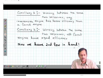
So, which is the corollary 1 in case of Carnot theorem. Now for the second part when which says the working between same 2 reservoir all Carnot engine will have equal efficiency.
