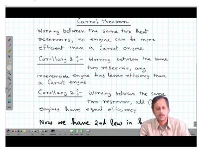
Carnot theorem I have just discussed in one of the previous lectures. That says working between any two reservoirs Carnot engine is the most efficient engine, yes and it has two corollary, one is working between the same two reservoirs an ordinary engine or a irreversible engine has to have lesser efficiency as compared to a idealized or Carnot engine or reversible engine.
