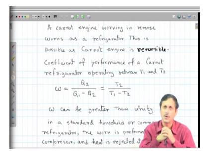
Now Carnot engine is a reversible engine as in all the processes are reversible. So, if we instead of using it as an engine if we just reverse the process, so that means it will absorb initially it will absorb heat from the cold reservoir and then isothermal compression will take place then it will have an adiabatic compression, finally it will reject heat to the hot reservoir.
