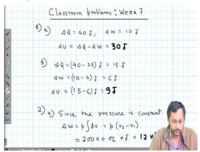
We have delta Q is equal to 40 Joules which is going into the system delta W is equal to 10 Joules which is work done by the system. So, this is also very important, it is said done, while the system does 10 Joules of work. So, 10 Joules is the work done by the system. So, dU = dW - dQ which is equal to 30 Joules. Now, for the next part, we have a transfer of 25 Joules out of the system, while 4 Joules of work is done on the system.
