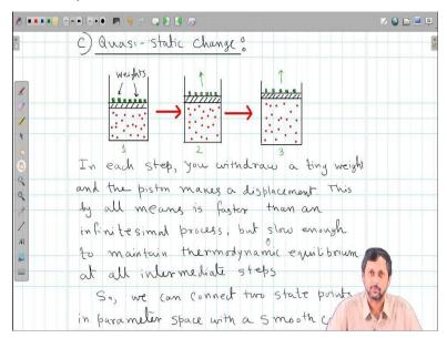
So, once again we take an example of a piston gas piston and cylinder arrangement. Let us say we have a certain amount of gas enclosed inside this piston and we have small weights placed on the piston ring on the piston plate. So, now this weight in the first position in this case position 1 this weight is exactly equal to the internal pressure. I mean it is sufficient to balance the internal pressure and there the piston is in a stationary position.
