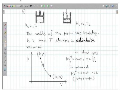
Now, if we do this compression for an isolated cylinder that means if we have a thermally isolated cylinder and we still compress it then not only PV but also temperature changes. So, we have PV T 1 P 1, V 1, T 1 and from there we go to P 2, V 2, T 2 and in this case, there is no exchange of heat energy with the surrounding. So, this process is called an adiabatic
