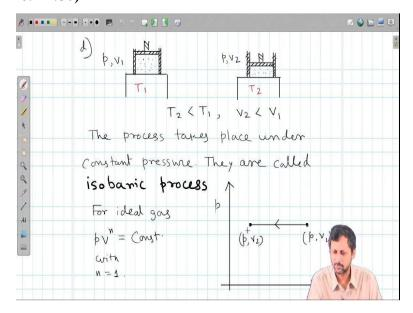
Similarly, if we now maintain the process the cylinder in, we change the temperature such that we maintain the pressure inside the cylinder. So, it is very simple if T 2 if the second heat was T 2 is less than T 1 then what happens the pressure drops and correspondingly sorry the so let us assume this pressure inside is just good enough to hold this cylinder or sorry the piston in a floating position.
