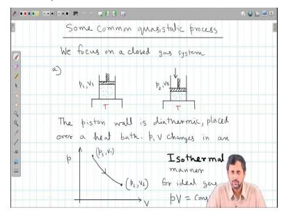
So, let us take some example some common example of quasi static processes which we commonly encounter in classical thermodynamics. The first process is let us say the cylinder piston arrangement we place that on a heat path and then we slowly compress it. So, when we slowly compress keeping it on a heat path and let us assume the wall of the cylinder is diathermic. So, that means heat energy can exchange.
