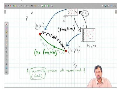
So, let us go back to this type I mean basically we talked about one such diagram where the process the system in our case it is a closed cylinder closed gas system inside of Piston cylinder arrangement. So, the initial state was sorry P 1 V 1 and then if we just let it expand then the piston will move out so the volume will increase pressure will drop so it will go to the second, another state which is given as P 2 V 2 on this PV indicator diagram.
