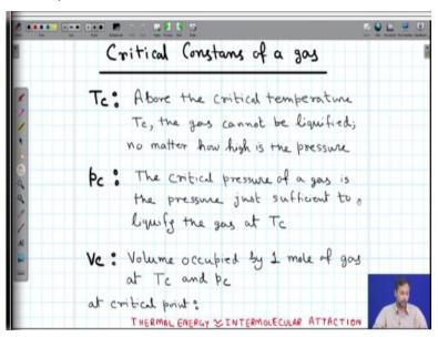
Next is and of course we learn about these critical constants of a gas. So, what are the critical constants? Tc is the critical temperature above which a gas cannot be liquefied, no matter how high pressure do we apply; pc is the critical pressure of the gas at which it is that the pressure which is just sufficient to liquify the gas at critical temperature. So, essentially this point here corresponds to the critical pressure and temperature.
