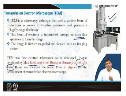
In addition, SEMs are able to give you, reasonable micrographs in the range of 40 nanometers or above. If you want to go to dimensions less than that, then you use FESEM's, which can give you reasonably acceptable quality micrographs in the range of 20 nanometers, plus/minus. But, if you want to go below that, then you need to go to transmission electron microscope. And this is a typical instrument of a transmission electron microscope.
