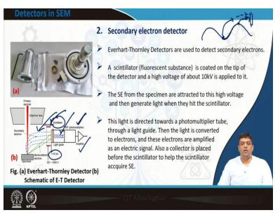
For(semi) secondary electrons you have a slightly different detector that is the Everhart-Thornley detector. This is a very simple design; the concepts are very similar. So, you have emission of low energy electrons, so then you have the potential which is able to attract these electrons which are emitted. Then you use a mesh, so you see that there is a mesh in the front of this detector. This mesh allows the secondary electrons to go through the opening.
