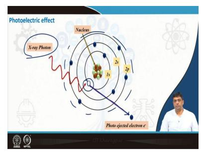
So, what do you have? You have the photoelectric effect. What happens, you have the X-ray photon incident on the sample; you have the nucleus surrounded by electrons. And because it is high energy X-ray photon, that is able to knock off the electron from the inner most shells or inner shells; so, you get information about the elements.
