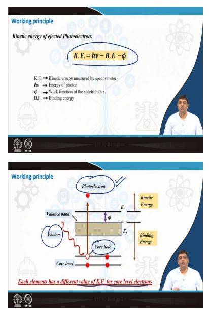
Working principle; again, just like photo electron or the photoelectric effect; you have the energy, which is given by hv minus the binding energy minus the work function of the spectrometer. If
