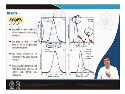
So, this is what a typical XPS micrograph looks like. So, I plot the intensity as a function of binding energy; so, this is basically the binding energy which is going to play the important role. For each element I know where the binding energy will lie. And then I can back calculate the element, which will be giving that binding energy.
