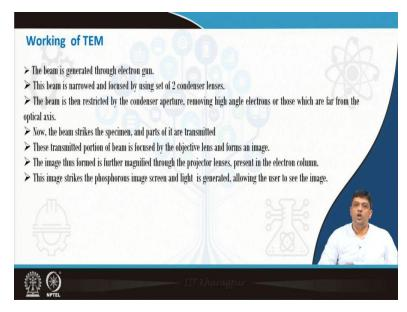
Very similar to what we had seen in SEM, you have the generation then the focusing. But, here the major difference is that once the sample is finding the electrons falling on them, the sample must allow the beam to go through. Or, you will must have signal in the transmitted region, and that signal is mostly analyzed to get the image.
