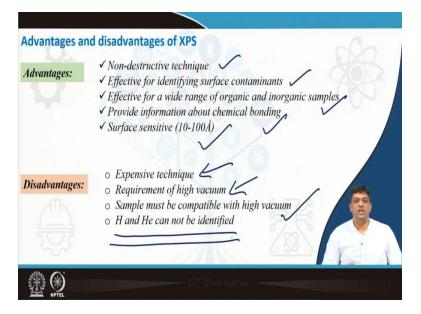
It is a non-destructive technique. It can be used to actually identify contaminants on the surface of a sample; large number of organic as well as inorganic samples can be investigated. It can give you information about the chemical bonding; and it is able to give you information about the surface. Again, with the techniques like XPS or the ones which we have discussed earlier today that is SEM and TEM. One factor gets associated, and that is they are quite expensive.
