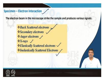
So, you can have back scattered electrons or secondary electrons, which are the two most used outputs of the specimen electron interaction. But there are other signals which can be obtained and analyze, you can get the auger electrons. You can get X-rays, you can get elastically scattered electrons, and inelastically scattered electrons. And then you will get auger spectroscopy or you will get excerpts on different kind of instruments are there, where you analyze these kinds of signals.
