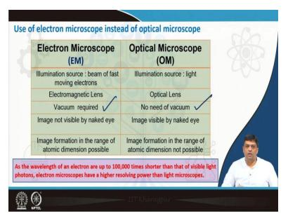
If you compare the two microscopes, then in electron microscope, you are using electrons as the fast-moving beam; whereas in optical microscope you use light as the illumination source. You can focus electrons using electromagnetic lenses; but for optical microscopes, you are using optical lenses. In the case when you have optical microscopes, you do not need vacuum.
