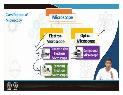
So, classification of microscope can be made. You can have optical microscopes, or you can have electron microscopes. Under electron microscopes, you can have transmission electron microscope or scanning electron microscopes. Scanning electron microscope, sometimes you also here FESEM that is field emission scanning electron microscope, is just the target of FESEM is changed; the target from where the electron beam is actually coming out. So, that is the major difference between SEM and FESEM.
