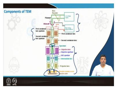
This is a typical TEM which is explained in schematic. So, what do you have? You have the generation of electron, you have the generation unit, then you have the focusing unit. You use the sample in the middle, and then you use the combination of various lenses to actually get the picture at the bottom. And you can see, you have started with a small region, but the image which you get is much more enlarged.
