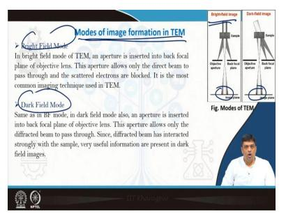
You can have various modes of operation of TEM, the bright field or the dark field; so, it depends on what type of beam you are using. So, whether you are using the direct beam to pass through and scattered electrons are blocked, or they are not blocked. So, depending upon what type of field or image you are constructing, you will have the two modes, and right field image mode is mostly used. And you at this moment, that is good enough for you to understand.
