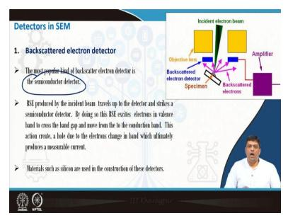
As we said, we in the back scattered mode you are understanding the elements above of the sample. So, you have various kinds of detectors, which are used in the back scattered electron mode; you have the detector, which is mostly a semiconductor-based detector. And in this, what happens when the electrons are received, then the electrons excite the valence electrons to the conduction electron.
