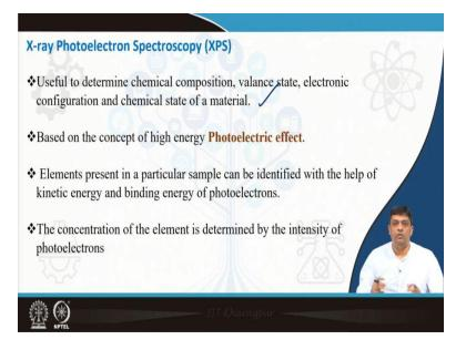
The final technique, which we have been using to understand the properties of nanomaterials, and I have mentioned earlier is XPS. This technique is basically high energy photoelectric effect-based technique. You can determine the elements which are present in the sample, you can find the chemical composition, you can find the valance state, you can find the electronic configurations, and you can also find the nature of interaction between the elements.
