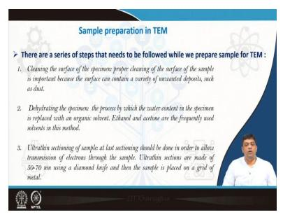
For making TEM samples, you must again clean the surface, you must have thin samples. You must not have samples which contain water, which can get evaporated in the column. If you have very large samples, then you must make it into three sections; and then that is done using the technique of (microtome). That is cutting of thin slices from a sample using diamond cutters, and that is called as (microtome); and this involves a trained manpower, because this is a non-trivial exercise.
