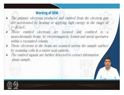
In SEM, you have the emission of electrons, either from electron gun which are accelerated, or by heating or by applying high energy in the range of 1 to 40 kilo electron volt. These emitted electrons are focused and then confined in a monochromatic beam of electromagnetic lens, and metal apertures within the vacuum column.
