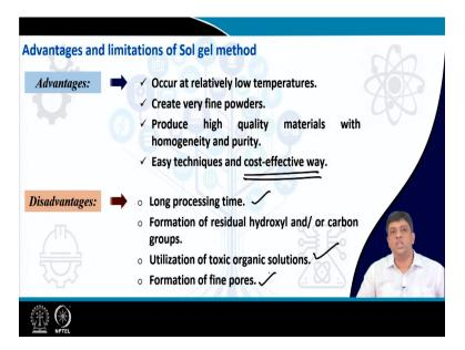
The advantages which are there with sol gel are, you are actually working at low temperatures. So, if you are working at low temperatures, then you can get fine powders and you can control the degree of agglomeration because even if you are making small particles, but if you allow all these small particles to come together an agglomerate then what you will see is a big chunk and that would appear to be a bulk big particular bulk sized system.
