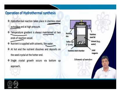
This is what you have, generally you use a stainless steel autoclave which is at which can sustain high temperatures and high pressure. There is always a temperature gradient which is maintained between two ends of the reaction vessel. So, once you have supplied the nutrients and then use some kind of a medium in which you can disperse these nutrients may it be water or any other kind of liquid medium so that you can ensure homogeneous distribution of these nutrients.
