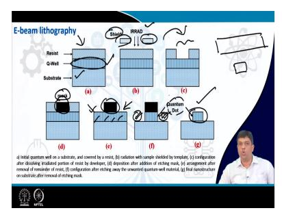
One of the most common technique used for top down process is the lithographic lithography you can have optical lithography, you can have electron beam lithography, or you can have iron
