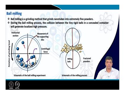
The next technique which you will use is most probably the ball milling technique, here you have a job where you have the balls inside. So, you can have very high grade steel or hard zirconium jars or if you are using softer materials like polymers, then you can have the jars made up of aluminium or so. And then what you do because of the collision between these balls which are inside the jars, then you crush the bigger size particles to smaller sized particles.
