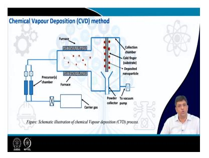
So, what you do you have the precursor chamber. So, you introduce precursors then they get heated in the furnace and then you introduce the carrier gas and using this carrier gas the carrier gas gets dissociated and then you can use the dissociated nucleus as the nucleating sites and from there you can lead to the growth of the materials which will go and get deposited on the substrate.
