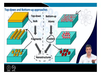
To understand these two protocols, let us have the two schematics to explain these two top down or bottom up approaches. The final aim is to get a nano structure. So, in top down approach, you already have the bulk material, what you do you actually reduce this bulk material to smaller fragments and then you go on reducing the size of the bulk material and what you obtain is the desired nano structure at the end.
