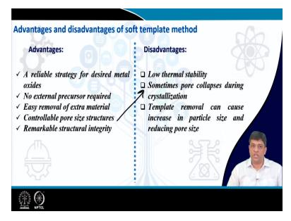
It has the advantage of reliability; you do not need external precursors. Easy removal of extra material that is a template can be removed, you can control the pore size by controlling the rate at which you are removing the template. But there are advantages which lead to disadvantage, here we said controlled pore size structure, but you can clearly see that sometimes because you
