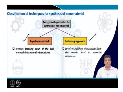
The synthesis protocols are broadly classified under two broad headings, the top-down approaches and bottom up approaches. The top down approach involves the breaking down of the bulk material into its nano size structure or the bottom up approach involves the buildup of a material from the atomic level and then scale up to the height of nano size structures.
