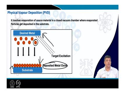
And similarly, to CVD, you also have physical vapor deposition techniques, which can lead to the deposition of nano structures on a substrate if you induce high energy beams on the design material, which gets ablated or are made to remove come out from the design material, then those materials will get deposited on the substrate in a pattern or a regular assembly or assembled order.
