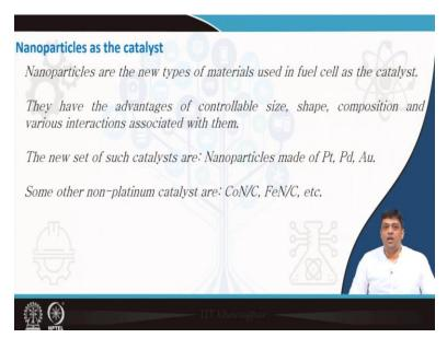
So, we have seen that platinum is mostly used, but then you need to have new materials which will replace platinum and with the advent of nanomaterials you can get large number of nanoparticles of various types of catalysts, which can actually deliver the performance that is desirable in a fuel cell.
