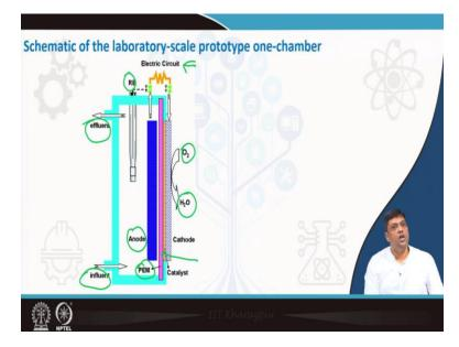
If you look into the design then you have the influent, the effluent you have the reference electrode, you have the external circuit, you have the catalyst loaded electrode. In addition, you have the proton exchange membrane, the anode. We are talking about the half cell. So, then you have the oxygen reacting with the catalysts and at the electrode, electrolyte interface and the output which you have is the water molecule. So, this is what you have as the prototype of one chamber.
