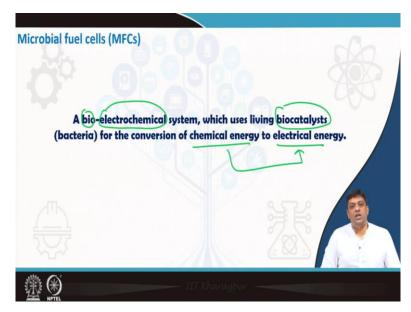
Broadly speaking, a microbial fuel cell is a bio electrochemical system which uses living bio catalysts such as bacteria for the conversion of chemical energy to electrical energy. So, you use living bio catalysts such as bacteria, which actually can take part in the redox reactions and then, because of that, you can get free electrons which can pass through the external circuit and you will get electricity.
