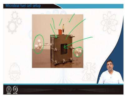
And this is what a typical fuel cell looks like, you have the outer plates, the screws, which are going across and tightening the two chambers, you have the air breathing cathodes, you have the way where you can control the flow of the influent or the effluent and then you have the reference electrodes or the nickel chromium wires for obtaining the electrons. And this is the other wire connecting the second electrode. So, this is a typical fuel cell which you can see.
