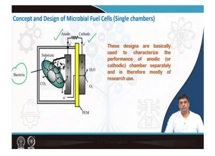
So, if you talk about single chamber fuel cells, you have the cathodes you have the anodes and you have the bacteria which is acting on the influent. What is the influent? Then that is the waste water or you use any solution or any waste stream collected solution where bacteria can act and then they can lead to the generation of electrons. This is what you are looking at.
