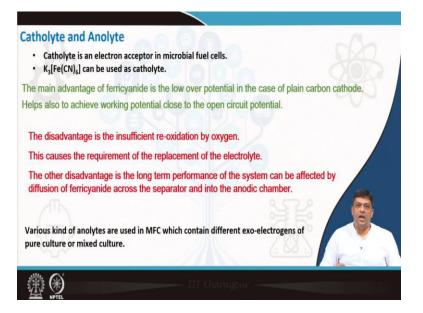
For example, let us take an example of potassium ferricyanide which is one of the commonly used catholyte. What is a catholyte? It is basically an electron acceptors. So, the main advantage of ferricyanide is it is lower potential in the case of plain carbon cathodes, it also helps to achieve working potential close to the open circuit potential or voltage. But there are disadvantages. So, it is insufficient re-oxidation of oxygen.
