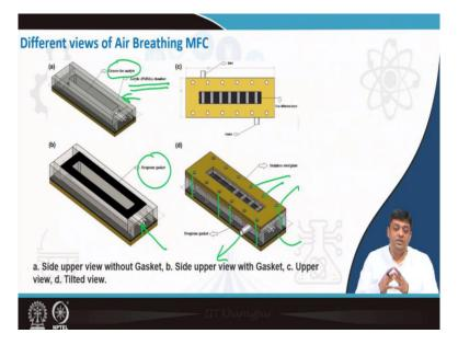
So, if you look into air breathing MFC where you are feeding air so, this is a typical design. What you have? You have the groove in the middle where you will have the anolyte then the whole chamber is actually made using an acrylic. So, you can why am I using acrylic because it is easy to mold and machine the acrylic based chamber.
