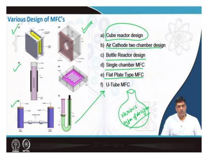
There are various types of fuel cells more so microbial fuel cells, which are used and the name actually comes in from the shape of the reactors. So, how does the MFC in given a, looks like? It looks like a cube reactor. So, it is called a cube reactor design of MFC or cube reactor type MFC. Then you have the air cathode but two chamber design, then you have the bottle reactor design, you have a single chamber MFC.
