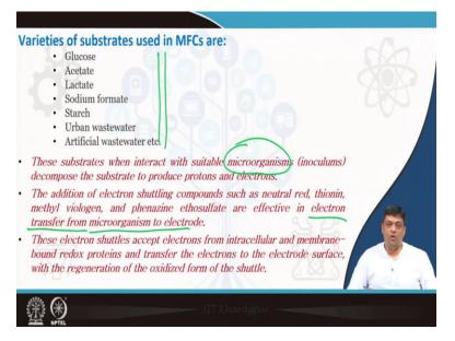
Varieties of substrates which are used in MFCs are substrates which will interact with the microorganisms. And the decomposition of the substrate will lead to the production of protons and electrons. So, you can use glucose, you can use acetates, you can use lactates or you can use wastewater, you can use synthetic wastewater, you can use starch.
