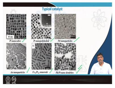
These are the typical catalysts which were initially used. Be it be platinum nanocubes, be it be platinum, nanopolyhedral type structure, be it be palladium or nanoparticles. But now, you can have gold nanoparticles, you can have a composite where you use iron with, with platinum or you can have any other kind of nano dendrites like structures made of palladium platinum composites.
