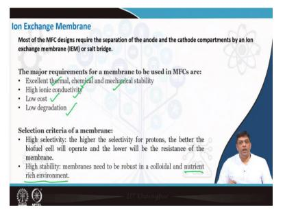
We have already seen the requirement of ion exchange or separator membranes over the last many weeks and the requirement of ion exchange membrane in MFCs are similar to what we discussed in earlier devices. They need to allow certain ions or protons to cross through and they do not allow the flow of electrons across them.
