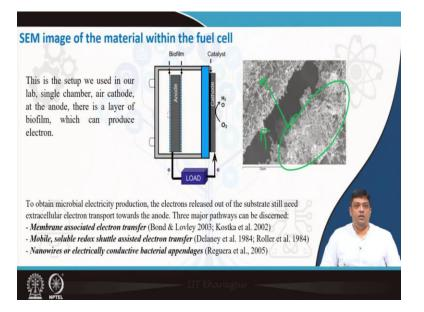
So, if you look into a fuel cell, then it must be clear to you, you will have membrane associated electron transfer, you will have redox shuttles taking part in electron transfer and for that you can use nano wires or electrically conductive bacterial appendages between the microorganism and the electron and that will ensure faster electron transfer.
