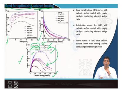
As we had seen earlier, once you have the design, once you have obtained the fuel cell, what will you do, you will obtain the polarization curves. The first measurement you will do is the open circuit voltage. The second measurement would be the polarization curves and then you will be plotting the power densities as a function of energy densities.
