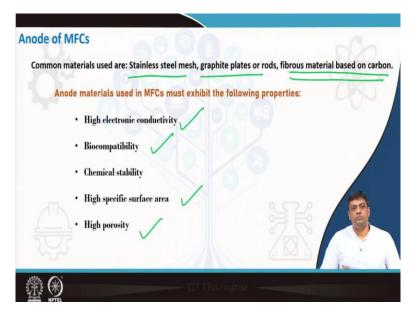
The common materials used in MFCs and let us say in anode side, is the stainless-steel mesh or you use graphite plates or rods or materials which are made up of different forms of carbon. But the properties you are looking at, in these materials are they should have reasonably high electronic conductivity, stability, both in terms of chemical and in terms of mechanical stability, because they will be exposed to harsh or toxic waste waters.
