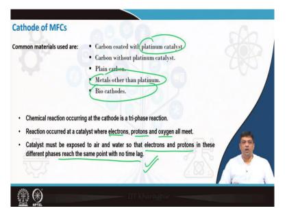
The cathode side, the common materials are based on carbon which are coated with platinum or any catalysts or you can have metals other than platinum which can also have the capacity to act as a catalyst or you can also have bio cathodes. The chemical reactions occurring at the cathode is a tri phase reaction and reactions occur at the point where electrons, the protons and oxygen's all meet.
