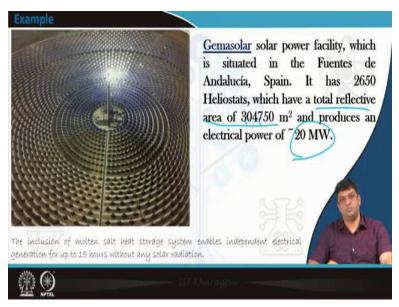
These are some of the examples which are there and are being used. For example, the Gemasolar in Spain with a total reflective area of more than 304750 meter square, is able to produce electrical power in the order of 20 megawatts.
