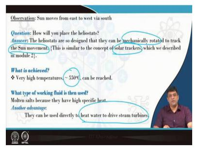
We know sun moves from east to west via south. What will you then be looking at? You are talking about how will you place these heliostats. You will place these heliostats so that they can be mechanically rotated to track the sun movement. This is the similar concept of solar trackers which we have discussed in module 2 and 3.
