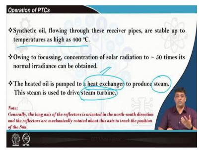
In addition, you will have to use heat transfer fluids which can sustain very high temperatures. Here we have talked about the use of synthetic oil which is flowing through the receiver pipes. And why are we talking about the use of synthetic oil, because they are stable up to temperatures as high as 400 degrees.
