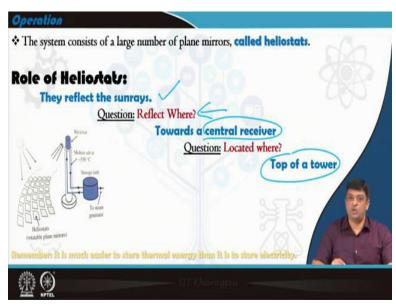
Hence, the role of the heliostats become critical, because they reflect the sun rays. Where do they reflect the sun rays? They reflect towards the central receiver. Where is this receiver located? At the top of a tower, and hence the name central receiver heliostats. Why this technology is becoming so useful, because it is much easier to store thermal energy than it is to store electricity.
