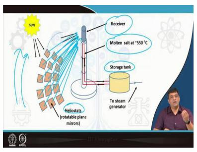
This is a typical schematic used to explain the operation of central receiver based on heliostats. You have heliostats, the plane mirrors, which can track the motion of the sun. So, you can track the motion of the sun. What are these mirrors going to do? They have to be so made that they, all these mirrors will reflect the solar radiation towards the receiver. This is what you are going to.
