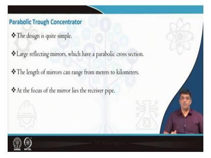
As I said, design is quite simple. You need large reflecting mirrors so that you can collect lot of solar radiation. These mirrors have a parabolic cross section. In reality and they have been actually investigated and installed in various test fields, the length of the mirrors can range from meters to kilometers if you are drawing the parabolic mirrors. And at the focus of the mirror lies the receiver pipe.
