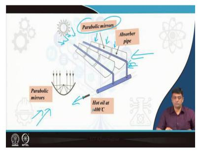
This is a typical design of a parabolic trough concentrator. You can clearly see what are they made of? They are made up of parabolic mirrors. Now, these parabolic mirrors are going to receive the sun rays and then focus the radiation on to the absorber pipes. So, they will focus the radiation on the absorber pipes.
