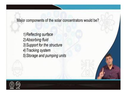
Major components of the solar concentrators would then be, you would have the reflecting surface, the absorbing fluid. Where would you install the whole structure? You cannot just let it lie on the ground. So, they have to be properly installed on a support structure which can also be used to have the inbuilt capacity of tracking the solar radiation that is the movement of the sun.
