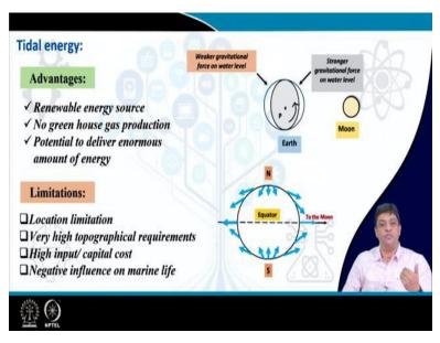
Which were the last two we had discussed, tidal and geothermal. So, in tidal energy, we all know tides, you were using high tides and then storing the water in a reservoir when you had high tides and letting the water flow through the turbine back to the sea when the condition of low tides was observed. But high tides, do you have high tides every time? No. That means you again have the parameter that is intermittent nature.
