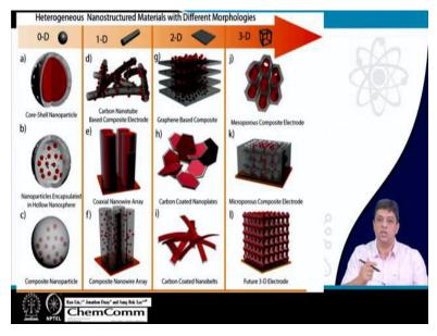
What do we understand by materials and nanomaterials? So, if you talk about bulk, then we mean that you have a system which is, let us say, three-dimensional structure and where all the three dimensions are having the values of more than 100 nanometers. So, nanomaterial is defined as the material which has at least one of the three dimensions in the range 1 to 100 nanometers. That is a typical definition for nanomaterials. So, you can have 0D, 1D, 2D or 3D structures.
