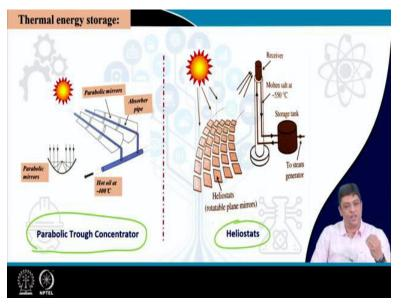
For the next example that is thermal energy storage systems, we will be focusing mainly on two types of systems, the parabolic trough concentrators and heliostats. The water heaters and the process of storing energy in a heat transfer fluid or using heat transfer fluids transferring heat to water or any other fluid that can be stored in a tank was discussed earlier and that is also considered as part of the thermal energy storage.
