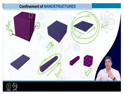
So, you can let us start with a 3D structure. So, you have an x direction, y direction and a z direction. So, if in all the three dimensions, the dimensions are more than 100 nanometers, then you have the bulk structure. Now, if you start cutting in, let us say, from the z-axis, so the second animation, so you have started reducing the size in the z direction, and you reach the point which is encircled now.
