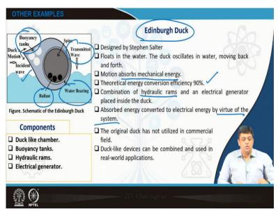
One of the earliest designs which were made by Stephen Salter to extract power, but a design which has not gone into commercial use is the Edinburgh Duck and this Duck has the design given in the left-hand side picture. So, you have the buoyancy tanks which are preventing this Duck to sink.
