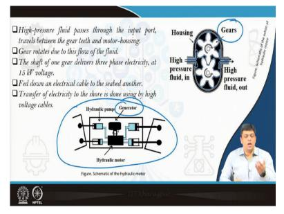
If you look into what I said, the hydraulic motors they are the typical structures which are shown here. So, you have the hydraulic pumps will take the water, through the water that will result in a hydraulic motor and you will have the generators. Once that is obtained the water will then come out and go to the next.
