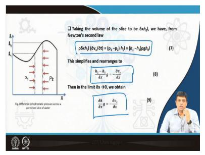
Now taking the volume of the slice to be del x  $h_0$  l, using Newton's second law we have the relationship which is mentioned in equation number 7. If you rearrange this equation, you will immediately obtain the condition which states that  $h_2$  minus  $h_1$  upon del x into g is equal to del  $v_x$  by del x. Then for the condition we are simulating that delta x tends to 0. What do we obtain? We obtain that del h by del x into g is equal to minus del  $v_x$  by del x.
