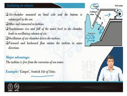
The second technology which is being developed is the oscillating air column devices. So, what happens? There you were sending in water inside, collecting it in a reservoir and then sending the water down to run the turbines. Here, the design is slightly different. You have the ocean waves which are moving in and in this, you install a structure which is similar to an air chamber mounted from the land side.
