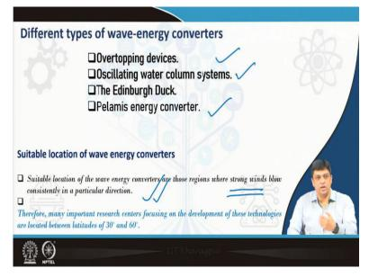
And there are different types of wave energy converters that are being installed and investigated. Some of them are listed in this slide, you can have overtopping devices, you can have oscillating water column systems, you can have Edinburgh Duck type structures which try to extract power from the moving wave or you can have Pelamis type energy converters.
