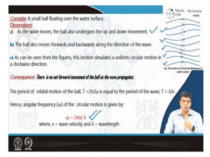
To understand this concept, let us take a water surface. On this water surface, you just have a small floating ball. So, I have put a small floating ball on top of this water surface and what are we doing? We are actually examining or monitoring the way this ball will move as a function of travelling water f.
