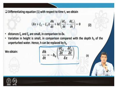
Differentiate that equation with respect to time and if you have the distances xi 1 and xi 2 which are small in comparison to delta x and you also know that the height changes which you observe are small, then you can replace h by  $h_0$  and what you will obtain that the change in height as a function of time can be written as delta h by delta t is equal to minus of  $h_0$  there xi 2 upon delta t minus t bar xi 1 by delta t by table delta x.
