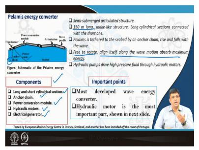
So, to counter these kinds of factors you have a new design which came into picture such as the Pelamis energy converters which are actually anchored. So, now you have the similar design but you have these structures are anchored, so that they do not flow away from the place they are installed.
