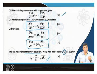
Again, differentiating with respect to x, you obtain another relation and if you differentiate equation 10 with respect to time, you can immediately write the terms such as del 2h upon del t square is equal to minus  $h_0$  del 2  $v_x$  by del x del t. We know the values in the earlier slide substitute them and you will get del 2  $v_x$  by del t del x is actually equal to g  $h_0$  del h by del x square.
