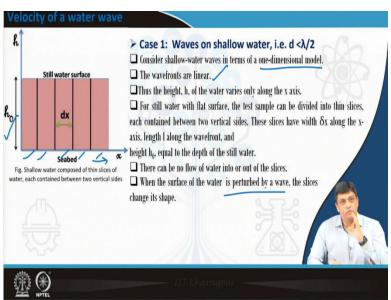
For this, let us try to start with case number 1, that is we are in the shallow water. So, consider shallow water waves and to simplify the model in terms of one-dimensional model just to simplify the picture. The wave fronts which are moving forward are considered to be linear. So, the wave fronts are moving in one direction and they are considered to be linear. Thus, what happens, the height h of the water varies only in the x direction for still water.
