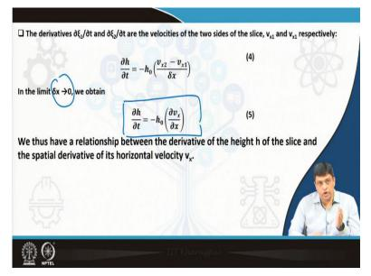
And in the limit, delta x tends to 0 we have a condition which will give us that delta h by delta t is equal to  $h_0$  delta v x by delta x. We thus have a relationship between the derivative of the height h of the slice and spatial derivative of its horizontal velocity that is  $v_x$ .
