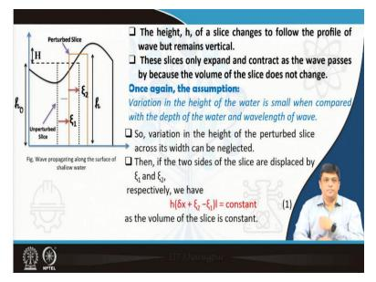
And then try to find out what is the value of velocity we can obtain. Now the height  $h_0$  of a slice changes to follow the profile of the wave but remains vertical. So, as the wave changes when I am at the bottom then the height changes, when I am at the top the height changes and that is why the height changes. These slices only expand and contract as the wave passes by because the volume of the slice does not change. So, once again what would be the assumption?
