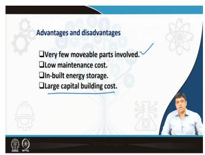
For example, you have large capital building cost. The advantages, it has very few movable parts, low maintenance and it has an inbuilt characteristic of energy storage. Why I have sent in water stored in reservoir. Now the energy is already stored in this water. The time I need energy, I will switch on the turbine and let the water flow down the penstock or the tube which is sending down the water to the turbines.
