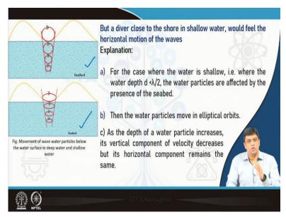
But the case is slightly different when you are at shallow waters. So, the water depth is less than lambda by 2 and here, the water particles are affected by the presence of the sea bed and if that happens that you are actually not able to reach this condition of nearly 0 amplitudes or radius going to nearly 0 value, the water particles move in elliptical orbits as you see from this picture.
