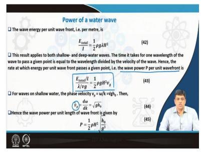
Now the wave energy per unit wave front that is per meter is what you have E total by l is equal to half rho g lambda H square. This result applies to both shallow and deep water.
