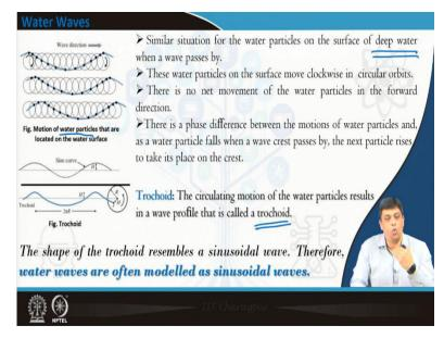
Similar situation actually is observed if you are monitoring water particles on the surface of deep water when a wave passes by. Deep water, you will understand what we mean by these terms in subsequent slides. So again, if I monitor the motion of water particles, the motion of water particles that are located on the surface of the water.
