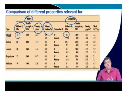
So, this table just gives you the relative properties between the fibers and the different types of composites be it be stiffness, be it be density. You will see that you get different kind of properties. So, for the commonly or routinely use glass, fiber glass E which is a low electrical conducting glass, you see the stiffness Ef has a value of 72 GPa in comparison if you talk about composites then the values may be quite different.
