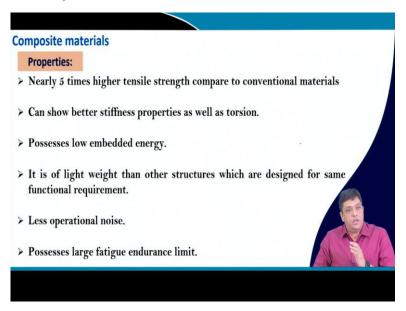
The important properties of these composites are they generally have 5 times higher tensile strength compared to the conventional materials. They show improved stiffness properties, they possess low embedded energy, and they also give you much lighter weight materials or structures but they maintain the required performance characteristics similar to those from conventional materials. And they also have higher fatigue endurance limits.
