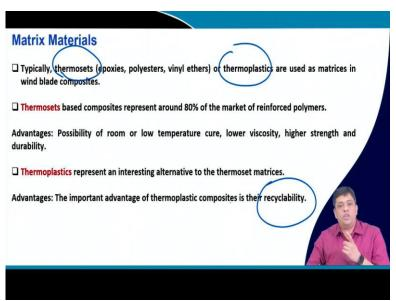
And finally you have matrix materials which are used in carbon fibers and typically thermosets are used or thermoplastics are used as matrices in wind blade components. Thermoset based composites actually as of today have 80 percent of the market of the reinforced polymers. Because they ensure lower viscosity, higher strength, they are more durable, and they can be prepared at room or slightly low temperature.
