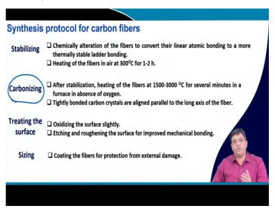
Stabilizing means that you are chemically altering the fibers to convert their linear atomic bonding to a more stable and thermally stable ladder bonding. And they are junk, for this process you heat the fibers in air. Let us say at around 300 degrees C for 1 to 2 hours. Once you have stabilized the carbon fibers you perform the carbonizing. For this, you take the
