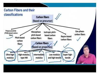
As of today the next class of fibers which I am mentioning those are based on carbon are mostly used and they have large number of applications and they are finding using various kinds of systems. The carbon fibers can be classified under various sub headings or based on the way they are synthesized or the shape and the size. So, let us say the carbon fibers if you just want to classify them based on the precursor which was used to fabricate these fibers.
