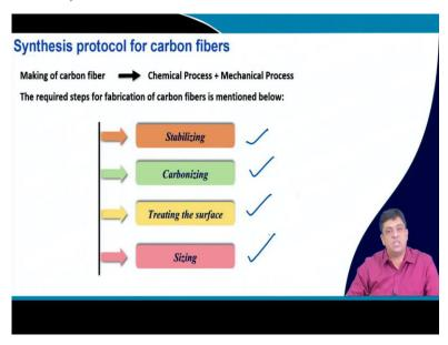
The question one must ask that if I am interested to work on these carbon structures and then use them in device, how do I obtain these carbon structures? Then mostly these carbon fibers are obtained with a combination of initial chemical process followed by a mechanical process. And typically the steps involved to obtain the carbon fibers include stabilization, carbonization of the precursors treatment of the surface and then sizing of the fibers.
