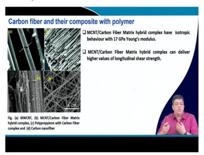
Similarly, you can see that you one can have different forms of these fibers. For example, figure a gives you the picture of a multi walled carbon nanotube that is MWCNT. So, single wall carbon nanotube you have arrangement with just in a way that you have a single tubular morphology. But if you have multiple tubes then running parallel to each other then you can call them as multi walled carbon nanotubes.
