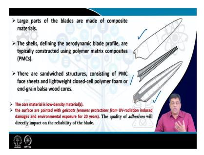
In the earlier lecture we saw that the wind turbine blade has shells, the two shells which are aerodynamic blades, they are brought together and in between you have a sandwich structure which consists of a PMC face sheets which are made of light weight close shell polymer foam or end grain balsa wood cores. The core of this blade is of low density material if I asked you this question, why do you need the low density material? Because we want to maintain low weight of the turbine.
