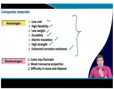
So, once again advantages low cost, high flexibility, low weight, they are more durable, mostly they are electrically insulating, while they are ensuring high strength, and enhanced corrosion resistance. So, if you talk about the properties which were required in a wind
