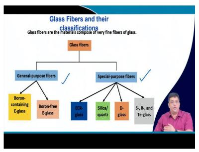
Similar to carbon fibers the other class of fibers which are useful to us are glass fibers. And then there are various types of glass fibers you can have general purpose glass fibers or special purpose glass fibers. But you will see that 90 percent of the fibers are general purpose fibers. And those are the ones which are used routinely in making composites or fiber base substrates.
