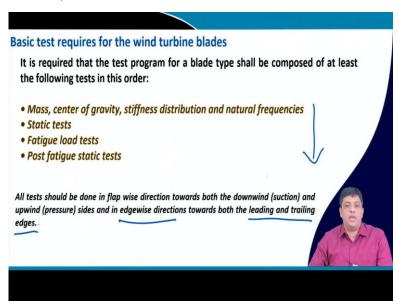
The basic tests which are required to certify or characterize the wind mill properties are the ones such as the mass, the center of gravity, stiffness distribution, or natural frequency based
