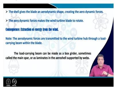
We had seen that the shell gives the blade an aerodynamic shape. Why do you need an aerodynamic shape? Because this shape leads to the appearance of the aerodynamic forces. These aerodynamic forces make the turbine blade to rotate. What is the consequence of appearance of this force and the induced rotation that you can extract energy from the wind. Because wind is leading to the rotation and if you are coupling your system with the electric motor then you can extract the energy.
