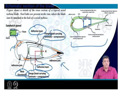
And we had seen the schematic of a typical wind blade which are used in today's wind turbines. And you see what do you have? You have two aerodynamic shells separated by the load bearing web and they are joined by various adhesives. So, you can see if you zoom this section you can clearly see that there is a sandwiched panel with the core and the faces in between.
