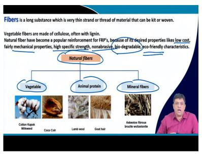
As indicated materials will be playing a critical role in giving you the desired performance. And there are different types of materials which are able to give you the desired performance. And the most important and relevant to us for this module are fibers, composites, and matrix materials. What are these three will be explained in next few minutes. Let us take the example of fibers. What are fibers?
