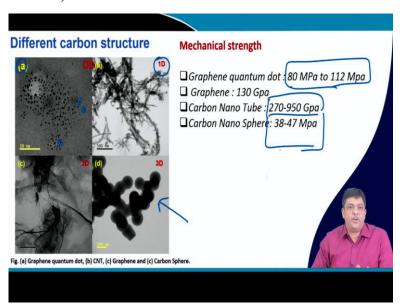
If you see the scanning electron microscope or the transmission electron microscope pictures which are shown on the left hand side of this slide you will see that there are different types of materials or morphologies or shapes of certain particles which are shown. Actually these are the different shapes of carbon structures or the structures which are formed using carbon itself.
