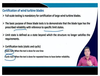
And these blades once they are fabricated using different types of materials cannot just be taken and installed in a turbine. They must go full scale testing and there is a certification process for wind turbine blades. And these blades are certified that they are able to give you the prescribed reliability and the specific limit states. And classification tests can be both static or cyclic. Static tests are what when the test is done for one time.
