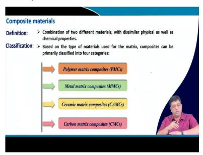
The next class of materials which are useful for wind turbine blades are the composite materials. These materials basically are obtained as a combination of two or more than two materials which have dissimilar similar physical and chemical properties. But when you bring them these two dissimilar materials together. The property you get from these mixture is very different from the individual properties of the materials which are being mixed together.
