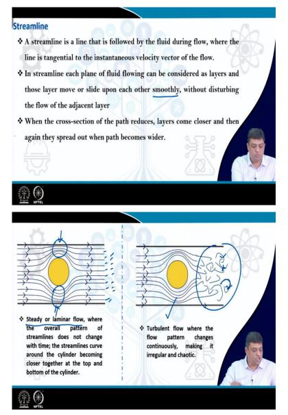
So, once again if you really want to repeat quickly, then a streamline flow is the one where the line is tangential to the instantaneous velocity vector of the flow and the fluid flowing can be considered as layers and these layers move or slide over each other smoothly without disturbing the adjacent layer. So, they even if they move they do not disturb the existing layer.
