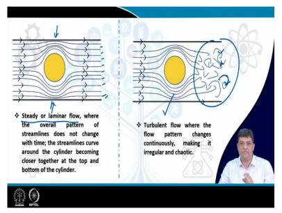
So, very quickly we will have more detailed discussions later on what is the difference between our laminar flow and a turbulent flow. So, if there is a flow and you put an obstacle in the middle, so, there is, so wind is flowing or fluid is flowing and I have put an obstacle. So, what happens to the flow, that is what we are talking about.
