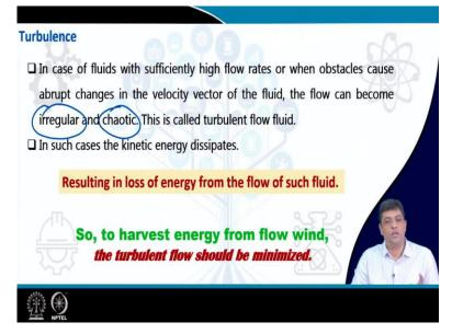
So, what happens in a turbulent flow. So, in case of fluid, which are having sufficiently high flow rates or when the obstacles in its path lead to abrupt change in the velocity vector, then the flow becomes irregular or chaotic or it is difficult to predict what will happen to the flowing fluid or the flow field once the fluid crosses the obstacle.
