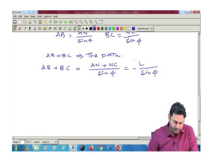
Now, what is AB plus BC? This is the path that is travelling by the light. So, this is the path that is travelling by this ray. Now, I can write this AB plus BC in terms of sin phi because I need to find out the relationship with this angle, whatever the angle it is making phi with the distance. So, AB plus BC is equal to AN plus NC divided by sin phi.
