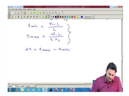
So, let me write t max once again in terms of refractive indexes. I just want to remove this sin phi. So, n 1 divided by L C sin phi is n 2 and I have n 1 square. So, this is my t max and this is my t min, these two are final expression. So, what is the delta t? So, delta t is the time lag between these two. So, I have t max, it should be t max minus t min.
