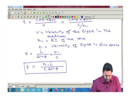
So, t that is the time that should take the path from go to A to B point through this A to C point through this reflection should be AB plus BC whole divided by the velocity. And we know the velocity inside a medium of refractive index n can be written as C divided by n 1, because n 1 is a refractive index and C is a velocity of light.
