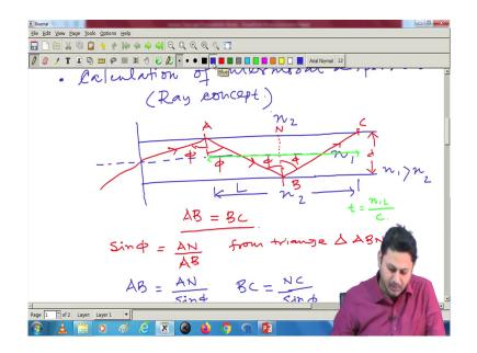
So, let us first draw the structure of the waveguide like this. This is the axis of the fiber core. This is n 1 – refractive index; this is n 2, this is n 2 – refractive index, where n 1 refractive index is greater than n 2. And if I launch a light here, let us make a different color, you will experience a total internal refraction like this, and hit here. Say this point is A, this point is B, this is C. This point says N, because I am going to use this point.
