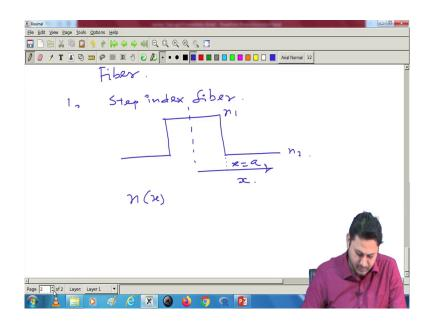
So, two kind of fiber refractive index profile I will going to mention today. And next class we will going to calculate something based on that. One is we already mentioned this one is step index fiber. For step index fiber, we simply have a step like structure like this. This is n 1; this is n 2. And along this we have say x; and this point is x equal to a.
