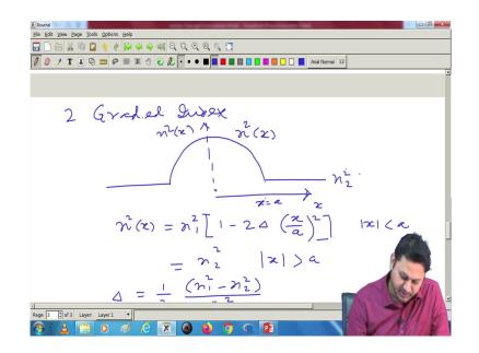
Another kind of refractive index quickly I like to mention which is graded index. In graded index, the refractive index profile has a variation like this - a parabolic kind of variation. This is the central part. This is along x.
