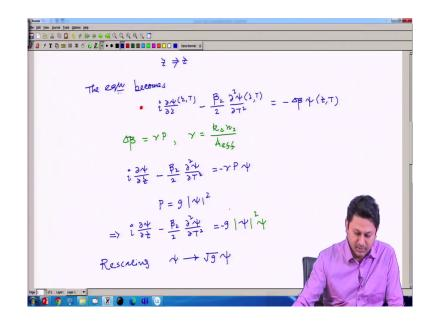
Now this power I can write in terms of psi. So, power is proportional to the mod of, so this proportionality constant I I can have like g, this we use this earlier also. This concept of the relation between P and mod of psi square. Well so, the equation then the equation becomes simply.
