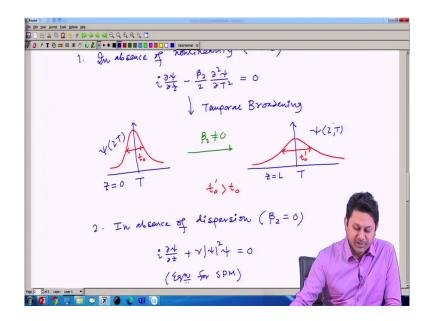
The governing equation of the pulse; that means there is no non-linearity, only dispersion is there. I am having this effects which is only the effect of dispersion. This equation basically tells us how the pulse will change under dispersion, and that we already know. And, as a consequence of this we have temporal broadening.
