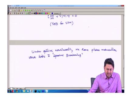
Under optical non-linearity we have phase modulation which leads to spectral broadening. So, the previous case when there was no non-linearity, only dispersion is there, we find there is a broadening and this broadening is; broadening was a temporal broadening. (Refer Slide Time: 28:33)
