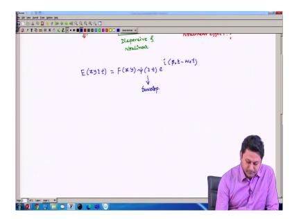
So, the total electric field we consider, whatever the electric field launch here, total electric field which is a function of x y z t, that we consider with this form, F x y. This is a transverse distribution. And then we have psi z t, which is basically the envelope which is changing with respect to time and also there is a z dependency, and the usual propagation term like this. Now, this is envelope.
