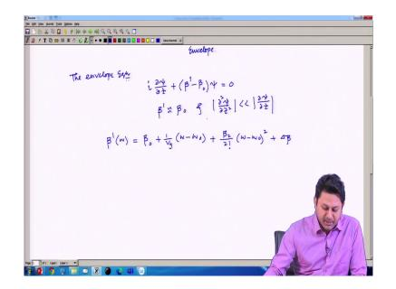
And from the Maxwell's equation, we derive the envelope equation. And, the envelope equation when we derive is come in now becomes like this become; the envelope equation becomes like this, under the consideration when the beta is nearly equal to beta 0. And also the slowly varying approximation was there.
