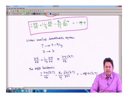
So, now, I have an equation after doing this operation I have i del psi del Z plus i 1 by vg then del psi del t. I just replace this omega minus omega 0 as an operator, i del l tau, then minus of beta 2 divided by factorial 2. Again, omega minus omega 0 square, I will going to replace as the second order derivative. So, it should be minus of this. And then psi and the right hand side I have delta beta psi.
