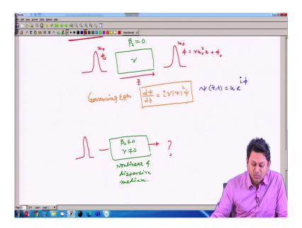
Now, today, in today's class let us modify this problem. The modification is I now I am having a waveguide, where beta 2 is not equal to 0 and gamma is as usual not equal to 0. So, the medium is non-linear and dispersive. So, now, beta 2 is not equal to 0. So, group velocity dispersion is no more 0.
