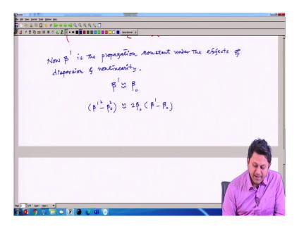
Well, that was the structure we have. And here we should mention that this beta prime, so, now, this beta prime is a propagation constant that contain. So, rather this is the propagation constant under the effect of dispersion and non-linearity under the effect of, under the effects of dispersion and non-linearity, under the effect of dispersion and non-linearity.
