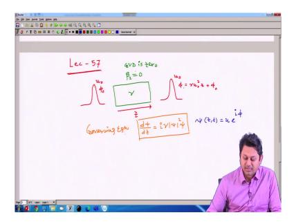
So, let us start with the concept. So, if you remember that in the last class, we tried to understand that if we have a waveguide defined by gamma and also I need to mention that there was no dispersion. So, group velocity dispersion is not there. So, beta 2 which is the defined which is basically, defined the group velocity dispersion is 0. So, group velocity dispersion is 0.
