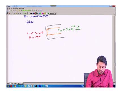
So, let us consider for conventional for conventional fiber; for conventional fiber. So, this is the fiber structure we have and we have a co-region here, and what happened that I launch an electric field with certain power. Let us take this power as normally, it is of the order of milli Watt normally, this is the this is the power we work with and then, the value of n 2 we know is 3 into 10 to the power of say, minus of 20 meter square divided by Watt.
