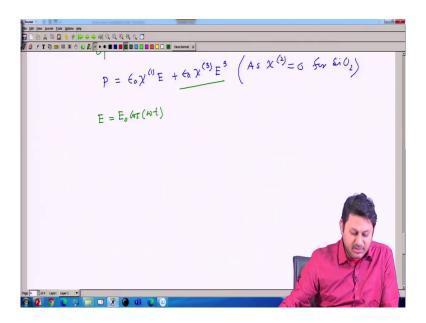
So, in optical Kerr effect; what we try to understand is this. So, P in fiber I can write in this form as chi 2 is 0 for silica. Silica is a centrosymmetric molecule. So, for centrosymmetric molecule, we mentioned that chi 2 is 0. So, since chi 2 is 0, we can say that my P is this quantity. I am not going to take the more higher order term I only take the first higher order term which is this one related to chi 3.
