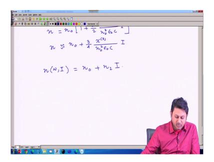
So, if I make a series expansion it should be n is nearly equal to n 0 plus 3 by 4 then, chi 3 divided by n 0 square, because one 0 will cancel out c and then, I. This expression I can write as n which is normally a function of omega now, become a function of intensity like I, is equal to n 0 plus n 2 I. This n 2 is called the Kerr coefficient.
