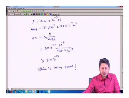
So, P is equal to 1 milli Watt given. So, this value is nothing, but 10 to the power of minus 3 of Watt. And then, A-effective is say, 150 micrometer square so, I can write it as 150 into 10 to the power of minus 12 meter square roughly. And then, delta n should be equal to n 2 then, P divided by A-effective this is the value of n 2 that is the change of refractive index due to the non-linearity. So, now, I will going to put this value whatever the value I have.
