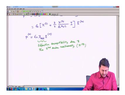
Then, what I do? I just rearrange this term and I have E 0 chi i plus 3 by 2 chi 3 divided by epsilon 0 n 0 c and then, intensity I and E omega. I can write this entire equation as P is equal to epsilon 0. And I write this term which is in the bracket as chi effective some chi effective and then, E, which is having the same frequency omega.
