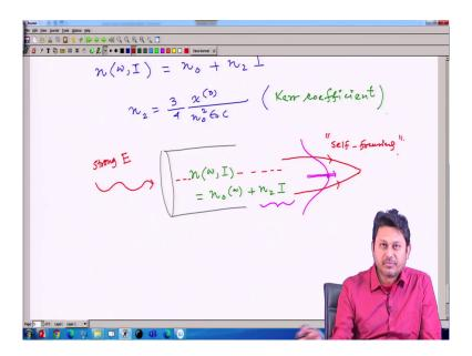
So, n 2 here is 3 by 4 chi 3 whole divided by n 0 square epsilon 0 c. So, this is called the Kerr co-efficient. So, here, we can see that the refractive index now, modified by the input electric field itself. So, if I have a waveguide or a say, fiber structure like this and if I launch a very strong electric field then, what happened the refractive index of this system.
