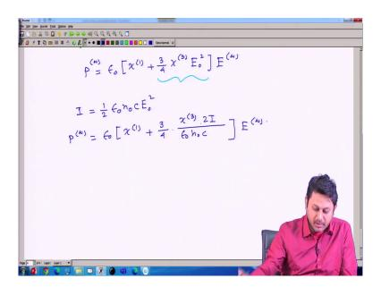
So, then what happened I can write the P in this way. So, my P here, the non-linear polarization term will be added to the P. So, I have the term P as which is a frequency of omega. In the right-hand side, all the frequency all the terms is having the frequency omega. So, I have chi 1 plus 3 by 4 chi 3 E 0 square then this E omega.
