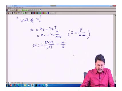
Unit of n 2, so, n I write this as n 0 plus n 2 I; I is a intensity. So, I can write it as n 0 plus n 2 in terms of power, it should be power divided by the effective area. As intensity can be represented as power divided by area a effective is a effective area. So, refractive index is a dimensionless quantity. So, from here, I can say that n 2 the unit of n 2 should be the unit of effective area divided by the effective (Refer Time: 23:05) the power of the system.
