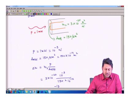
And one parameter is required that is A-effective. So, A-effective is of the order of say, 150 micrometer square. This is roughly the value for a fiber standard fiber. So, now, let us calculate, because all the values are there.
