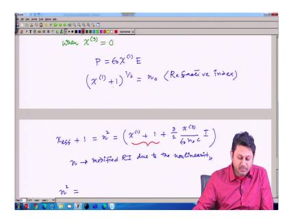
So, in absence of non-linearity so, when chi 3 is equal to 0, there was no non-linearity. I can simply write my P as epsilon 0 then, chi 1 and then E and from that I can write that chi 1 plus 1 whole to the power half; that was the refractive index of the system that was the refractive index of the system.
