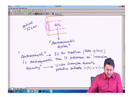
So, for optical fiber now let us go back to our old very old structure of optical fiber that this is a cladding and inside the cladding we have a portion which is core. And now this fiber is made of silica. So, it is made of silica. So, it is essentially SiO 2. So, this is optical fiber. So, optical fiber is made of silica and this silica has a special property. This silica it is a special property, it is a centrosymmetric molecule, it is silica centrosymmetric molecule.
