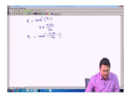
So, R which we figure out as tan hyperbolic square then kappa L, it can be written as so, kappa so kappa we also find out that it is this roughly nearly equal to when the operating wavelength is very close to the value of the brag wavelength then, this reflectivity can be simply written as tan hyperbolic square pi delta n divided by lambda B multiplied by L.
