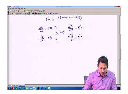
And also from these two equations coupled equation and decoupled and we had a differential equation for A and B individually, which is this.
