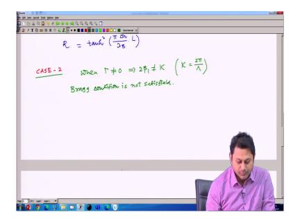
When so, this case 2 is the case, when this is not equal to 0 that means, the phase matching condition is not there anymore so, 2 beta 1 is not equal to big K mind it big K is 2 pi divided by lambda the grating period. So, that means, the Bragg condition is not satisfied Bragg condition is not satisfied.
