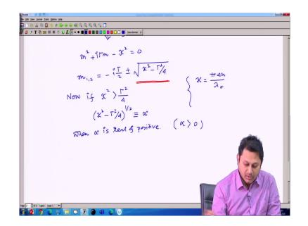
Then, it should be differential equation should be m square plus i gamma m minus kappa square equal to 0. So, the value of m say m 1, 2 there will be two roots of this equation and 1 can write this 2 root as this, which we use several time this technique so, it should be ok. So, this is the two roots this, these are the two roots m 1, 2. Well, now we assume so, we have something here very interesting which is kappa square minus this gamma square divided by 4.
