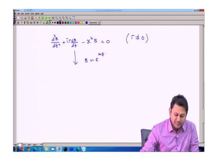
So, this simplify the equation as so, eventually I have a differential equation, and then minus kappa square B is equal to 0. After that so, this is the this is the condition and definitely when gamma is not equal to 0 goodness to say. Now, I should use this technique that I want to have a solution of the form say e to the power of mz.
