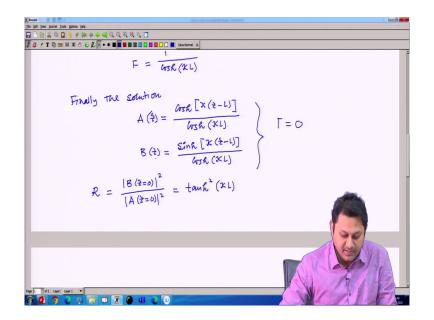
Then, the value of F I can write simply 1 divided by cos hyperbolic of kappa L. So, cos hyperbolic a kappa L is a constant. So, I can write the value of this constant F in terms of the coupling coefficient coupling constant kappa and the grating length L. So, finally, the solution that we had was A Z as cos hyperbolic of kappa Z minus L divided by cos of hyperbolic of kappa L.
