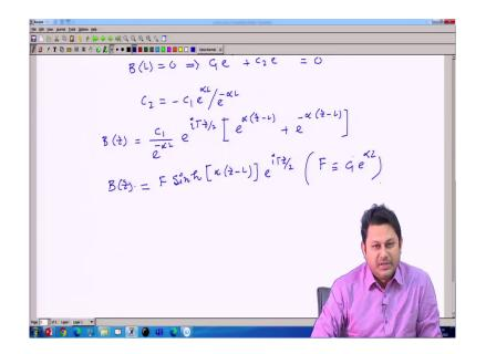
This thing I can write as F of sin hyperbolic alpha Z minus L into e to the power of i gamma Z divided by 2, when F is another constant, which I can write as C 1 e to the power of minus L.
