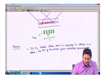
So, if I draw here only the core region, so this will come like this. Variation of the refractive index, the permanent damage of the refractive index here in the core region and I will going to have a grating structure. This is roughly the grating structure.
