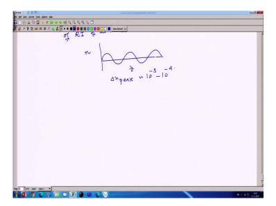
So, there is a periodic variation of the core, there is a permanent periodic variation of the core. So, there is a periodic kind of variation refractive index variation of the core as a function of z because of this interference pattern. I already explained that in this figure.
