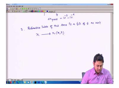
Next, what happened? The refractive, now the refractive index of the core is a function of z as well. That is important. So far we are dealing with refractive index as a function of x, but now this refractive index will be a function of x as well as z. So, that will give something extra in the couple mode theory.
