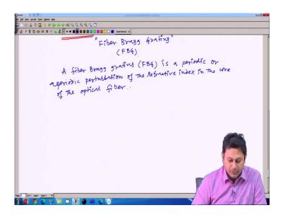
So, a fiber Bragg grating or in short FBG is a periodic or periodic or aperiodic perturbation of the refractive index in the core of the optical fiber. So, I try to draw this. So, what is the meaning of periodic or aperiodic perturbations that we need to understand. So, let me draw quickly the fiber structure.
