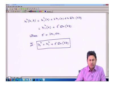
So, if I write all this whatever the definition now I write, with the whatever the definition I used based on that I can write n square which is a function of x, z is equal to n 1 square this is a function of x plus 2 n 1 which is a function of x. Then, delta n sine of K z or n 1 x square plus this entire term I write sigma, sigma of sine K, z. I will going to use this expression of n square in the calculation. So, that is why I just define this. So, when sigma is equal to 2 of n 1 delta n.
