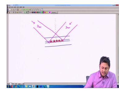
So, suppose this is the fiber and this is the core part of this fiber, this is the core part of this fiber. So, the fiber is placed in a in a field in a in a UV radiation, two lights, UV light is now allowed to fall over the fiber. And when these two light is falling over the fiber there should be some kind of interference of these two lights and because of that we can have some kind of interference pattern here. So, let me draw this interference.
