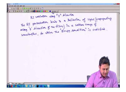
So, what happened? The refractive index, so what happened? The refractive index perturbation whatever the perturbation I put here, the refractive index perturbation on RI perturbation leads to leads to a reflection of light propagating along say z direction of the fiber. So, this light is propagating along z direction of the fiber.
