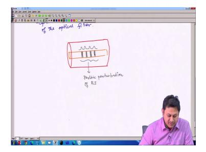
So, in the fiber we have a structure like this. I have a core part and I have a cladding part. In the core part, if I have a periodic variation of the refractive index like this. So, I have a refractive index n 1 of the core and n 2 of the cladding that we know. On top of that I now I am putting some kind of periodic perturbation in the core region along z direction. So, this is a periodic perturbation of refractive index.
