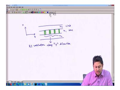
So, if I draw a straight forward simple two-dimensional figure, so this is the cross sectional view. So, I am having this. And I am having this perturbations here with certain periods. The same figure I am drawing, but in two-dimension and in the rest of the lectures, I will draw this two-dimensional figure, so that now you can realize in three-dimension what is the structure and two-dimension how it is changing.
