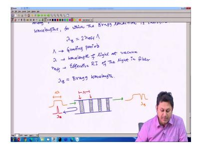
So, which wavelength will going to reflect back? It is lambda B equal to 2n effective we will going to prove that and big lambda, where this big lambda is the grating period and lambda is a wavelength of light at vacuum.
