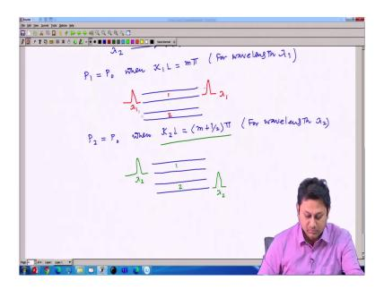
So, this is for wavelength lambda 1, so this is the value at which in the branch 1, I have entire power. So, this is the coupler, and I have lambda 1 here. So, there will be transfer, but the output I can have my lambda 1 here, because this is branch 1, and this is branch 2.
