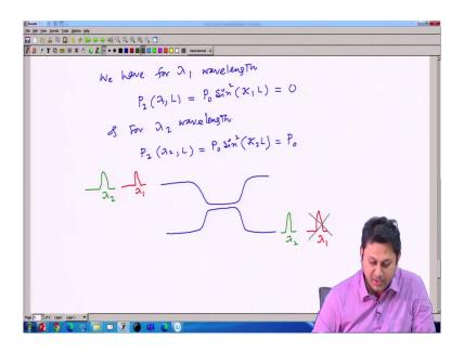
So, let me write it here. So, we have, so we have for lambda 1 wavelength, P 2 lambda 1 at some distance L is equal to P 0 sin kappa 1 L to be 0, that means, I do not want any kind of wavelength at output at second P 2 means at second branch. And for lambda 2 wavelength, I can have P 2. So, this is lambda 1. This is lambda 2, L equal to P 0 sin square kappa 2 L equal to P 0.
