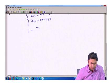
So, L, I can extract which is pi divide if I just make this minus this, so it should be simply. So, ok let me do that clearly. So, I can have kappa 1 minus kappa 2 L is equal to simply pi by 2. So, my L, the critical length at which these two wavelengths will be separate it out should be 2 of kappa 1 minus kappa 2.
