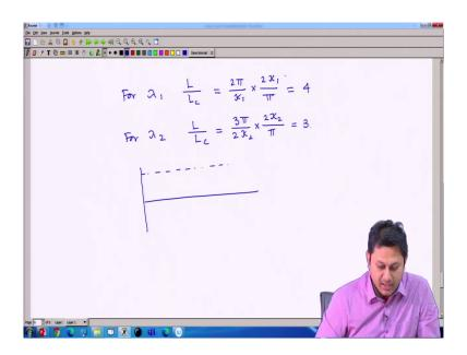
So, what about for lambda 2? For lambda 2 this value L divided by L c which is equal to 3 pi divided by 2 kappa 2 multiplied by 2 of kappa 2 divided by pi which comes out to be 3. So, that means, if I draw this stuff it should be something like that. So, this is the total coupling length.
