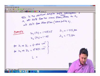
So, we quickly write down the example. So, one example, so consider a coupler with identical fiber such that say n 1 for lambda 1 is equal to 1.4525, and n 2 which is for lambda 2 is equal to 1.45. So, the refractive index of lambda 1 is this, and refractive index of the lambda 2 is this.
