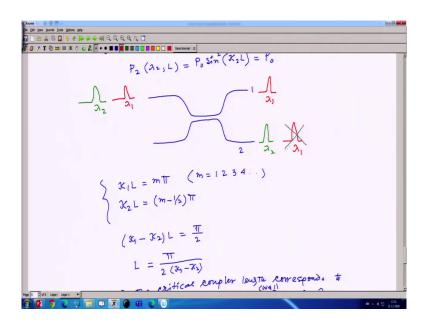
So, this condition if I look carefully satisfied when kappa 1 that length L is equal to m pi say m equal to 1, 2, 3, 4 so on. And simultaneously kappa 2 for the same length it has to be m minus half pi. So, from these two expressions, one can extract what is the value of the L.
