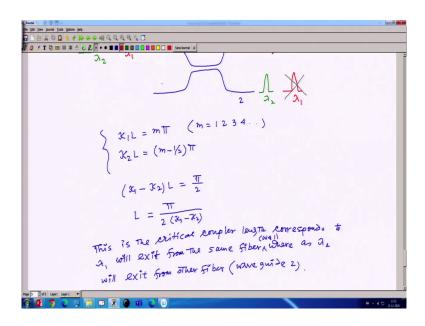
So, this is, so this is the critical coupler length corresponds to the fact that lambda 1 will exit from the same fiber where as lambda 2 will exit from other fiber. Other fiber means waveguide 2; same fiber means waveguide 1. So, I already draw that, that if this is waveguide 1, and if it is waveguide 2, so lambda 1 will going to come here, and lambda 2 will be here.
