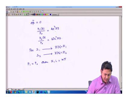
If I put delta beta equal to 0, then P 1 the expression will be simpler. So, P 1 divided by P 0 should be equal to cos square of kappa z, and P 2 divided by P 0 which is a function of z is equal to sin square of kappa z. Now, I mention that kappa is a function of lambda. So, for lambda 1, for lambda 1, kappa should be equal to kappa 1; and for lambda 2, kappa should be equal to kappa 2.
