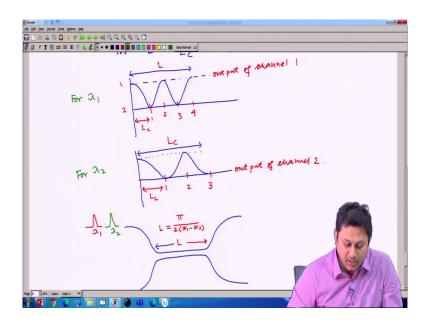
So, I have this total length of the coupler which is L. So, this is 1, and this length is my L c. This is another length 2, this is another length 3, and this is another length 4. So, you can see this is channel 1 and this is channel 2. So, output, this is the output of channel 1. This is the output of channel 1. What about and for lambda 1; as well because this is for lambda 1. So, this is for lambda 1.
