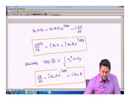
And the simpler form I can have is this kappa 11, after defining that A which is a function of z, then kappa 12 beta z; then e to the power of i delta beta z is equal to minus of i dA dz.
