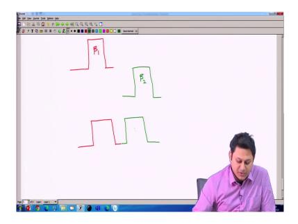
So, initially suppose I have one waveguide and I have a propagation constant beta here. Then I have another waveguide, individual another waveguide and this is beta 2. Now, what happened that, I now I have both the waveguides,, sorry let me draw in a logical way.
