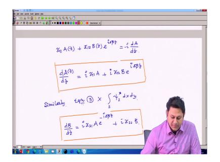
And the simpler form I can have is this kappa 11, after defining that A which is a function of z, then kappa 12 beta z; then e to the power of i delta beta z is equal to minus of i dA dz.
