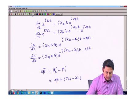
So, eventually I can have d a d z is equal to i of kappa 1 2 Bz e to the power of i kappa 2 2 minus kappa,, sorry it is kappa naught K; so kappa 2 2 minus kappa 1 1 z plus delta beta z. In the similar way, exactly in the similar way one can have d b d z is equal to i kappa 2 1 a z e to the power of minus of i kappa 2 2 minus kappa 1 1 z minus delta beta z.
