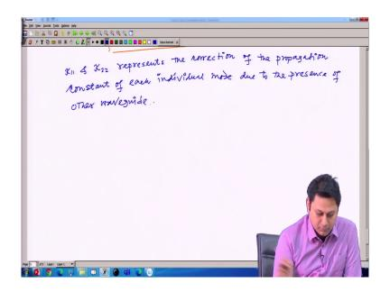
So, kappa 1 and kappa 2 is essentially. So, let me write down, kappa 11 and kappa 22 represents the correction of the propagation constant of each individual mode due to the presence of other waveguide. So, what was that?
