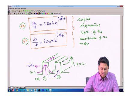
So, eventually I have a equation which is having the form like d a d z, which is a pure amplitude term is equal to, is evolving following this differential equation; then Be to the power of i delta beta tilde z. And this is one equation, so let me put in a bracket; say equation 6a. And another equation for b I have say 21 ae to the power of i delta beta tilde z,, say this is equation 6b.
