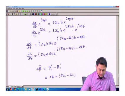
So, eventually I can have d a d z is equal to i of kappa 1 2 Bz e to the power of i kappa 2 2 minus kappa,, sorry it is kappa naught K; so kappa 2 2 minus kappa 1 1 z plus delta beta z. In the similar way, exactly in the similar way one can have d b d z is equal to i kappa 2 1 a z e to the power of minus of i kappa 2 2 minus kappa 1 1 z minus delta beta z.
