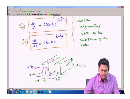
So, eventually I have a equation which is having the form like d a d z, which is a pure amplitude term is equal to, is evolving following this differential equation; then Be to the power of i delta beta tilde z. And this is one equation, so let me put in a bracket; say equation 6a. And another equation for b I have say 21 ae to the power of i delta beta tilde z,, say this is equation 6b.
