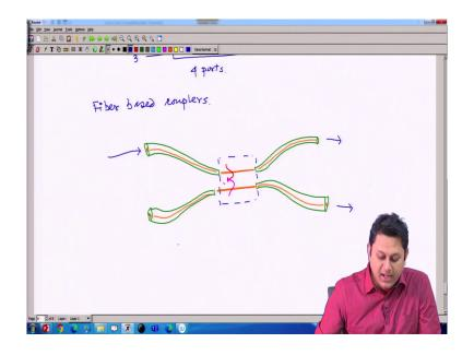
Well, normally the most popular one is the fiber based couplers. In the fiber based couplers what happened that ok let me draw quickly that I have a fiber like this cut here and inside that I have a core so, this is basically my core of the fiber and I have this and then again from here.
