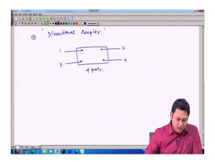
So, next try to understand the physics of the working principle of say directional coupler. So, definitely the name suggests that some coupling is associated with that and this coupling is essentially the light coupling so, I can couple the light from one web guide to another web guide and as a result we can have we can use this kind of this kind of system to different applications; and we will going to discuss this application in brief here.
