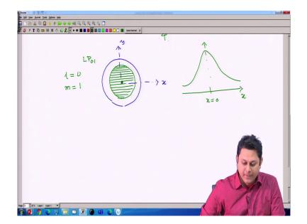
This mode is LP 01; that means, 1 equal to 0 and m equal to 1. If I want to find out the distribution over x-axis, this distribution will be something like this over x-axis. So, the intensity of the mode will be maximum here in the axis and then it goes like that. So, this is at x equal to 0 point. So, this is the distribution we have.
