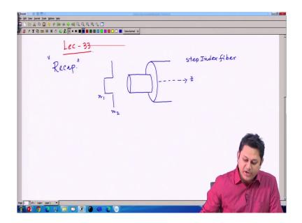
So, it is recap, a quick recap. So, this is the structure of an optical fiber, this is the core part and this is the cladding part, this is the geometry, this is z, co-refractive index is n 1 and cladding is n 2 for step index fiber. So, this is a step index fiber. So, we try to find out the modes in step index fiber which is a simpler one.
