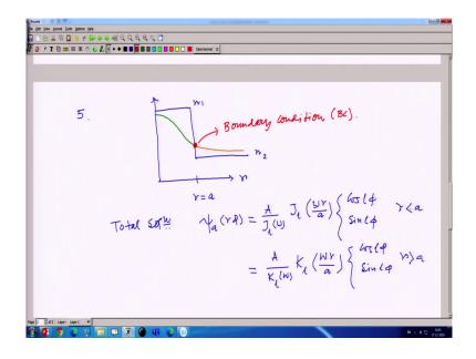
And, if I plot this solution then as 0.5 we did it. So, this is the fiber structure. We had a refractive index n 1 here and refractive index n 2 here. This point is r equal to a and along this direction is my r and the field is something like this. This is for equation 1 and another part this is for equation 2. Equation 1 means here this one first x square d 2 R dx square this equation the solution is given here, the green one and the orange one is a solution of this.
