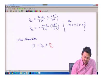
At least this is my 1.5 to 2.5 this equation works well. So now I have 2 dispersion, so let me now so the total dispersion eventually, if somebody want to calculate the total dispersion I can write D as a total dispersion and now it should be the combination of two dispersion one is waveguide dispersion and plus another is the material dispersion, which we already calculated in the previous class. If I add these two then I will go to get the total dispersion, now what is the material dispersion?
