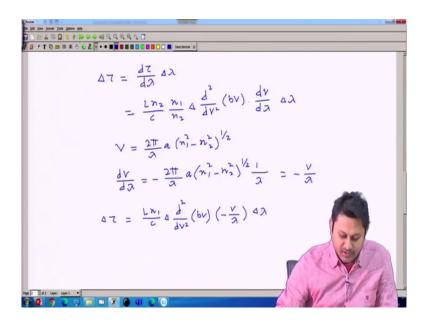
So, change of t which is delta tau equal to with respect to the wavelength, this calculation we already done in calculating the material dispersion I have to do that.
