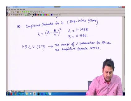
So, we can introduce the empirical formula for b, this is for say step index fiber true for, step index fiber and this empirical formula reads like this, where a b are constant and the value is precisely given as 1.1428 and b is 0.996 these are the two constant value of the two constant and b is x the form of b as a function of v is given in explicit manner, so that I can do the derivative.
