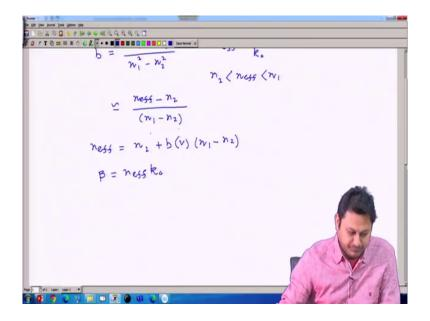
So, this equation can be approximated as n effective minus n 2 divided by n 1 minus n 2, well from that I can find out n effective as n 2 plus b function of v. In the last class we find that b is a normalized propagation constant and it should be a function of v, with changing v we find that b will going to change. Now, beta already I defined in terms of n effective it should be n effective multiplied by k 0.
