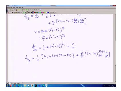
Now, v we know v parameter is defined as k 0 a n 1 square minus n 2 square whole to the power half by definition. Now I can write it as omega divided by c a n 1 square minus n 2 square whole to the power half. So, d v d omega this I can figure out and it turns up to be 1 by c a n 1 square minus n 2 square whole to the power half, I can simply write it as v divided by omega.
