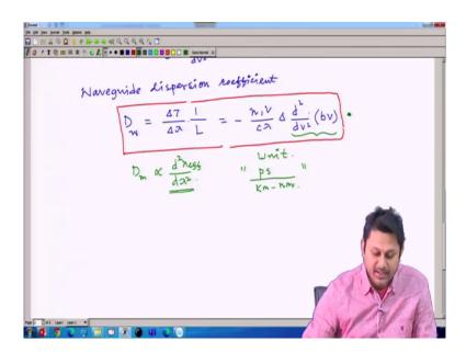
So, the waveguide dispersion coefficient the waveguide dispersion coefficient I write it as D w, for material dispersion we defined as D m here we going to define at D w, which is the same definition that rate change of tau with respect to the change of wavelength with unit distance.
