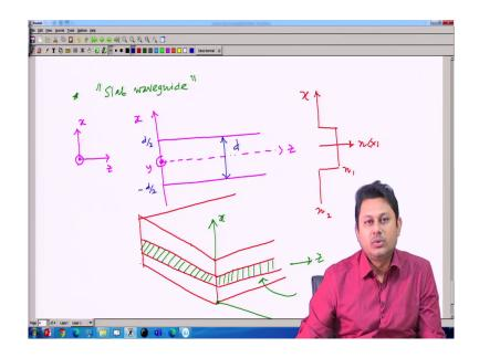
So, so, we will try to calculate the field distribution or the mode distribution in a slab waveguide. The slab waveguide already we define; this is nothing new. So, I have a refractive
