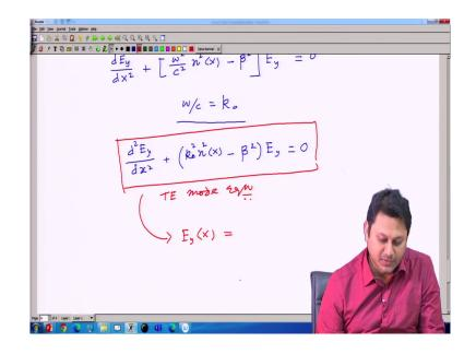
So, eventually I have a differential equation in this form d 2 E y d x square plus k 0 square n square x minus beta square E y is equal to 0. So, this equation is my mode equation for TE
