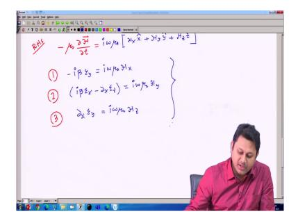
So, let me write equation 1. And if I tally the x-component, it should be simply because here I have the x-component i beta. So, I will just going to write that. So, minus of i beta E y because this is my x-component here that is equal to; that is equal to i of omega of mu 0 H x.
