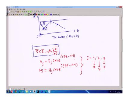
So, what are the equations? So, let me write down the equation. The first equation is curl cross E is. So, let me write once again curl cross E, first I want to execute this is mu 0 minus of mu 0 del H del t ok. And E j, the jth component of the E vector we define that in the last class, it is defined in this way. This is defined in this way.
