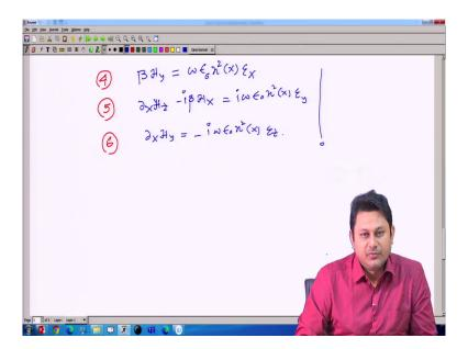
So, I have equation four as equating the x-component whatever we have in two equations here i beta and this. So, I have simply beta H y is equal to let me see what we have I have i will minus i minus a cancel out. So, it should be omega epsilon 0 n square. So, omega epsilon 0 n square as a function of x and E x that is my equation 4.
