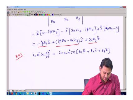
So, I can also simplify or just rewrite the x-component as ok. Let us write in this way minus of i beta H y x that is the first term, second term is plus of i beta H x minus del x H z y and then finally, plus del x H y z. So, I have the components, here this one and this one. This is my left hand side. I also should have expression in the right hand side.
